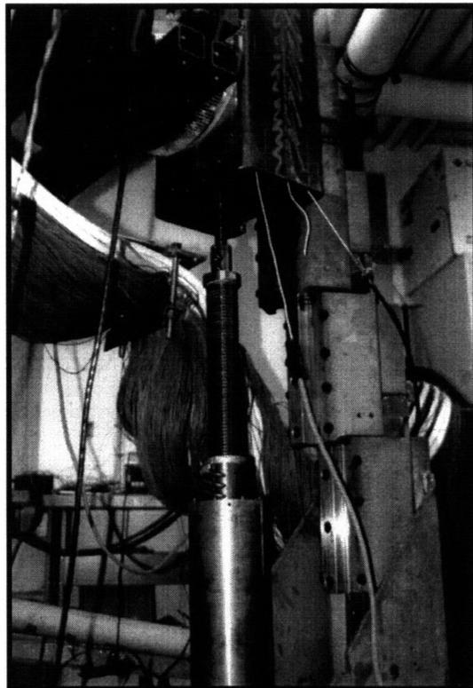
**Figure 3.15: Photograph of Alpha Prototype with Telescoping Ballscrew**
