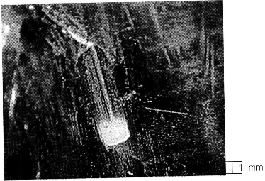
Crack initiation at the tip of the notch (A1)
