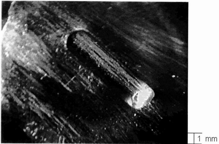
Multiple cracking in the notch and crack initiation at the notch end at the plate surface (B1)
