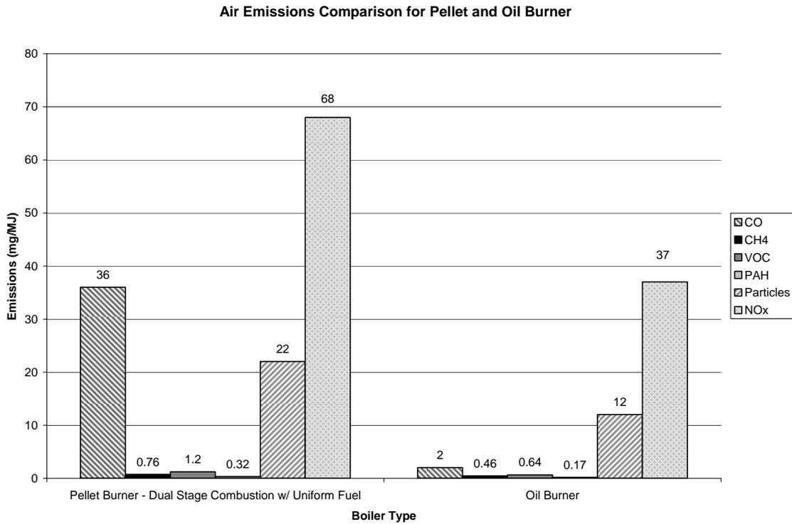
**Figure 15: Combustion Emissions Comparison between Wood Pellet and Oil Burners [Johansson, 2004, p4188]**
