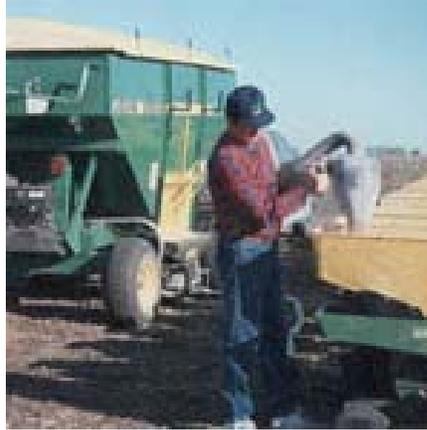
**Figure 13: One Person Handling the "SeedVac" to Transport Grain at Over 180 kg/min Through a Flexible Hose [Christianson, 2007]**
