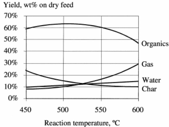
Typical yields of organic liquid, reaction water, gas and char from fast pyrolysis of wood, wt% on dry feed basis.
