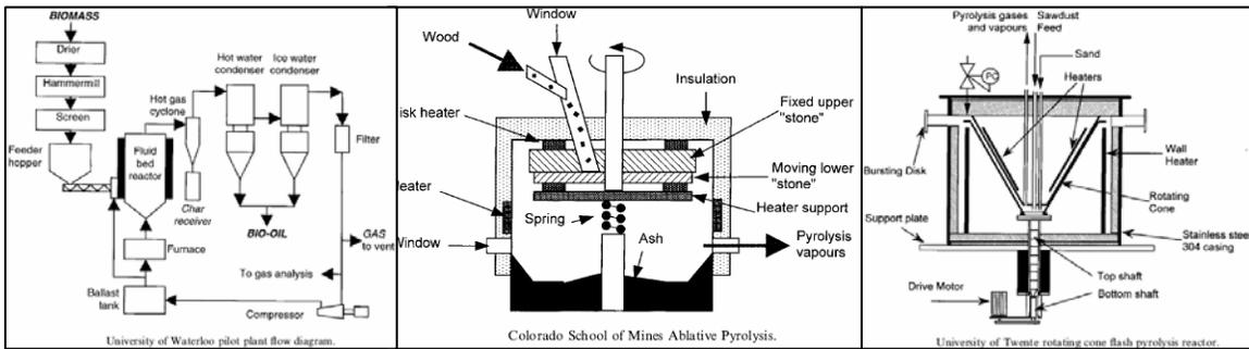
**Figure 12: Pyrolysis Reactor Types: Fluidized Bed, Ablative, and Cyclone (from left to right)**
