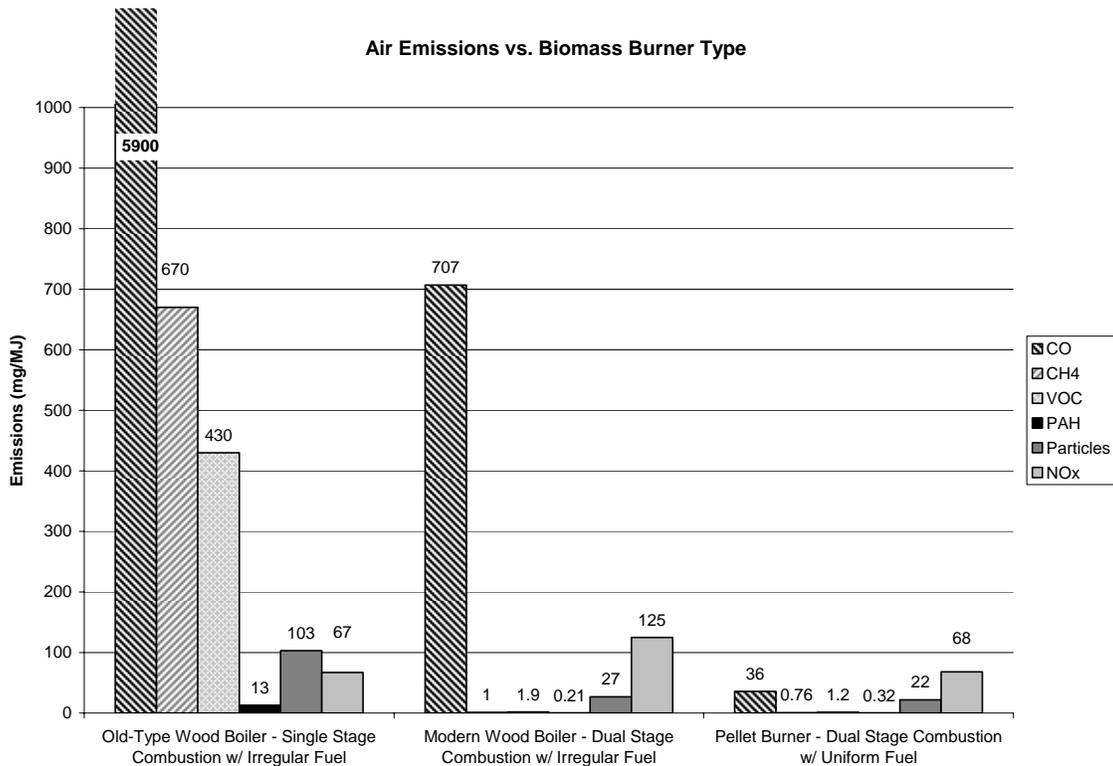
Figure 14: Combustion Emissions for Various Burner Types in Home Heaters [Johansson, 2004, p4188]
