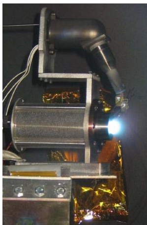
Figure 4-2: MHT-9 Hall Thruster in operation inside the MIT-SPL vacuum chamber
