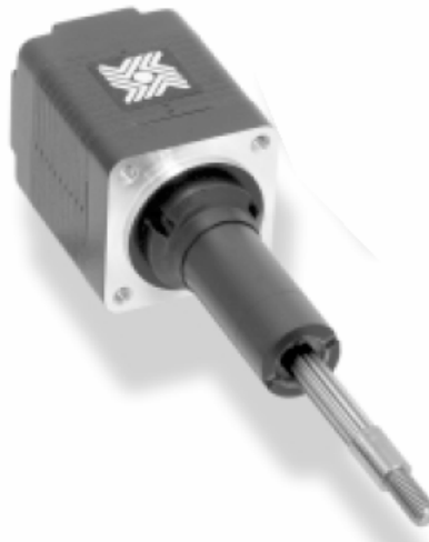
Figure 3.5: The Haydon hybrid captive shaft linear actuator is capable of a 1.5 um step size with a 9 mm stroke and thrust of 44.5 N [8].
