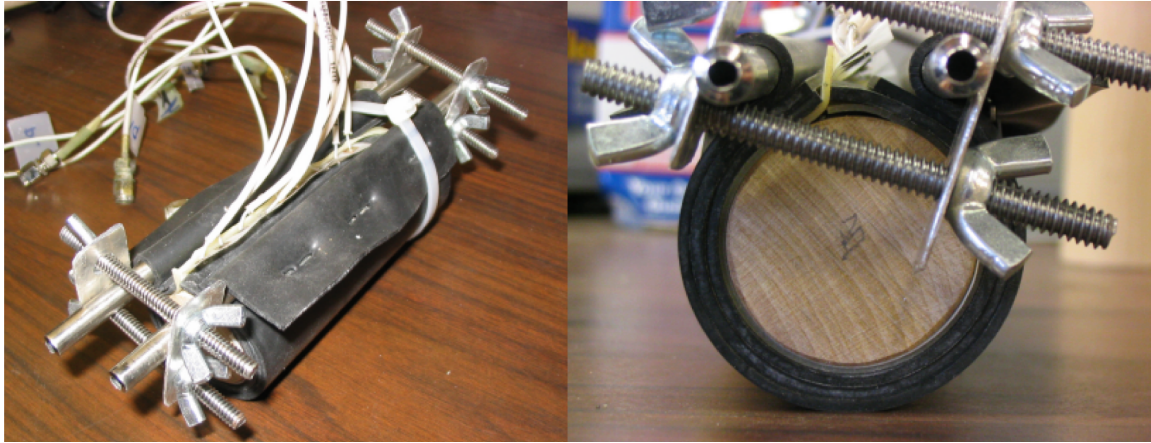
Figure 8-26: Photographs of a birch rod in the sling clamping mechanism with a z periodic sensor. The tightness of the clamp is adjusted by the wing nuts. Several layers of rubber are used to protect the sensor and limit the exposed area to the front surface.
