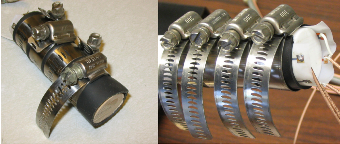
Figure 5-4: Photographs of the hose clamping mechanism for birch (left) and Teflon (right) sample setups.
