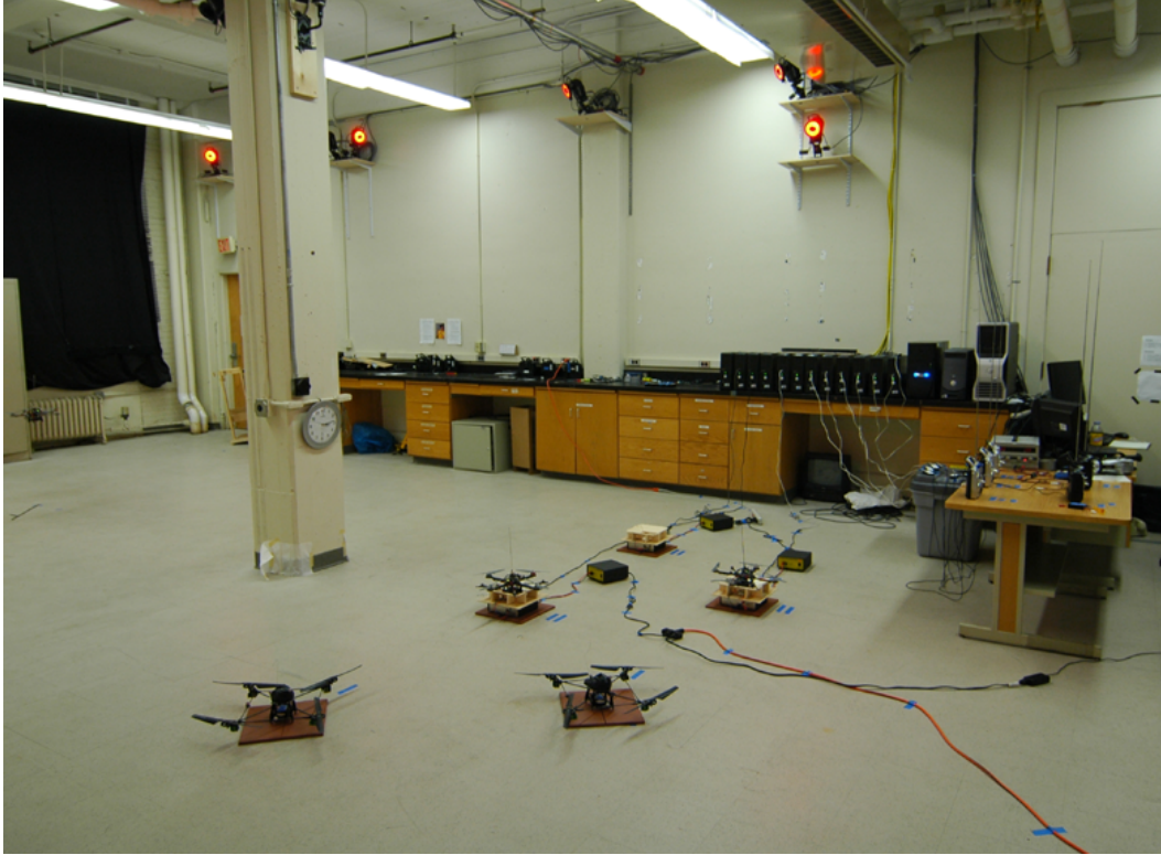
Figure 6-14: Automated 1.5 Hour Persistent Surveillance Mission (PSM) using Mission Manager with Basis Function Generation Algorithm with Five Autonomous Vehicles
