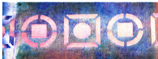
Figure 5.14. Photograph of patterned porous [(PAH 8.5/TPAArVBA 3.5) 10 -(PAH 8.5/PAA 3.5) 5 ] 3,5 film. 2 Regions with alternating porous/non-porous stacks show visibly uniform reflection, while fully porous regions show heterogeneous reflection [159].
