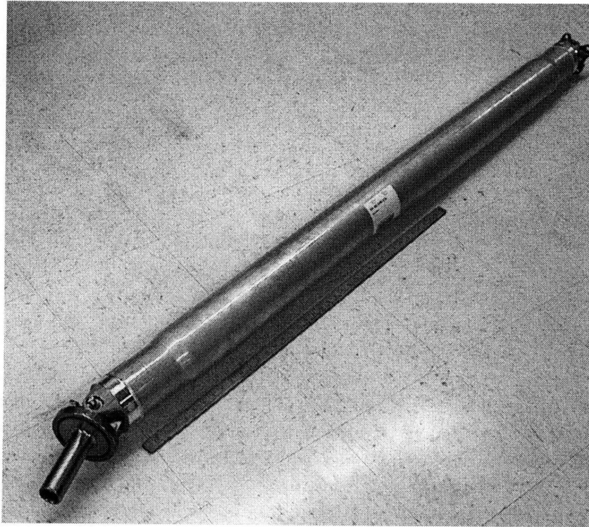
Figure 1-6: Photograph of a driveshaft (shown next to a meter stick for scaling)
