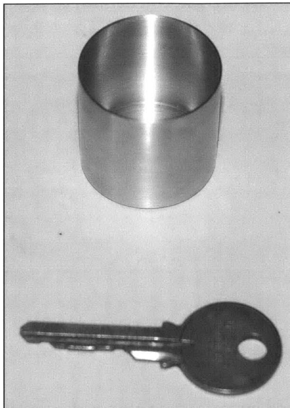
Figure 4.3: At 33mm in outer diameter, the HAMTA1 evaporation chamber (pictured here with a key for scale) was machined of aluminum to accommodate the DuPont porous membrane samples; 60mm x 45mm was the only size membrane available.
