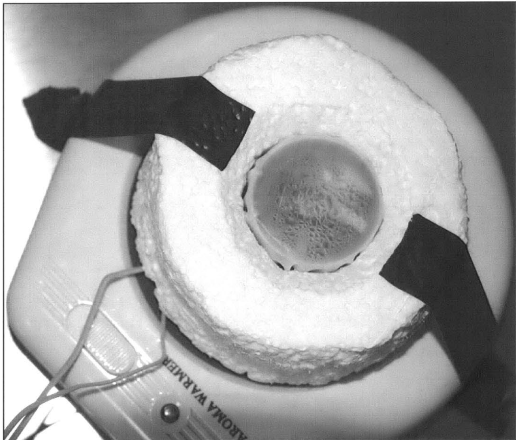
Figure 5.8 Liquid water droplets forming on the upstream membrane face during HAMTA1 steady-state operation result from use of buoyancy-driven natural convection, which was employed intentionally to eliminate complications associate with the moving evaporation front.
