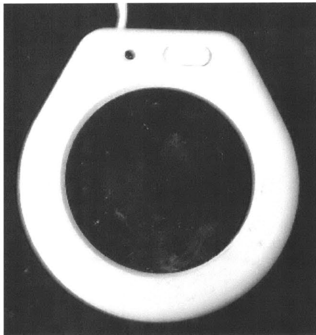
Figure 4.5: A commercial candle warmer provided input heat flux for the HAMTA1 evaporation experiments. Photo by the thesis author.
