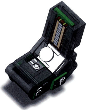
Figure 45: (a.) Squiggle series linear actuator; (b.) Ring Sensor using miniature piezo actuator.
