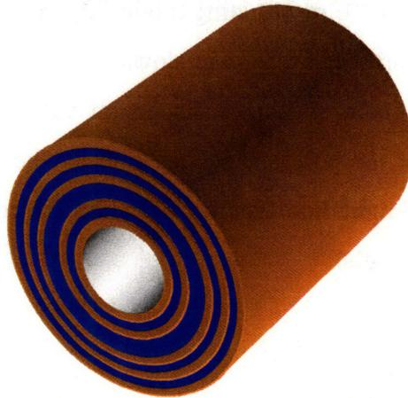
**Figure 1.8:** PBG fiber with a double thickness layer of the high-refractive index glass forming a  $\lambda/2$  defect state.
