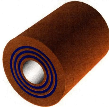
**Figure 1.2:** Hollow-Core Photonic Bandgap Fiber (PBG) constructed from two alternating materials with large refractive index contrast forming an omni-directional reflecting cladding that confined light with frequency inside the bandgap to the core region.
