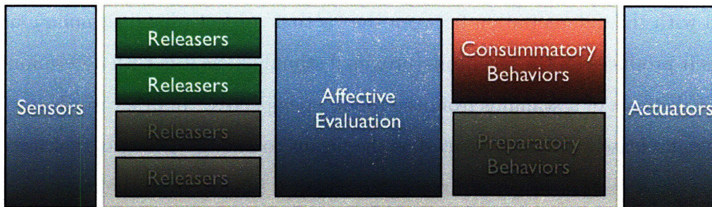
Figure 7-8: Pathway for Preparatory Behaviors. This figure illustrates the main organizational principle for action in the proposed framework as it relates to the notion of a separate sensorimotor pathway for preparatory or anticipatory behaviors that help the organism prepare to deal with environmental contingencies.
