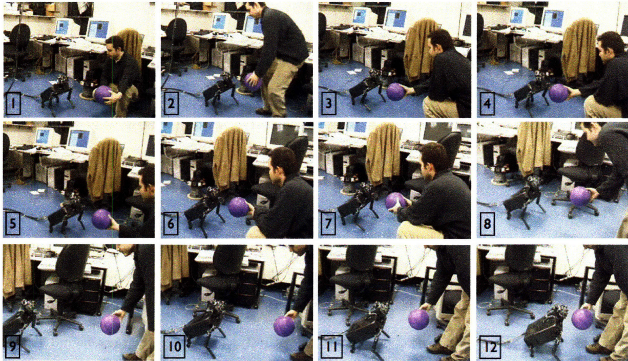
Figure 7-9: Distal and Proximal Releasers. This sequence of frames illustrates how the distal and proximal releasers that are used in Seeking Affect Program work. Distal releasers detect affectively significant stimuli at a spatiotemporal distance and send that information through the preparatory pathway, as described in the text, triggering an approach behavior until the significant stimulus is within certain pre-determined range, in which case the approach behavior is stopped.
