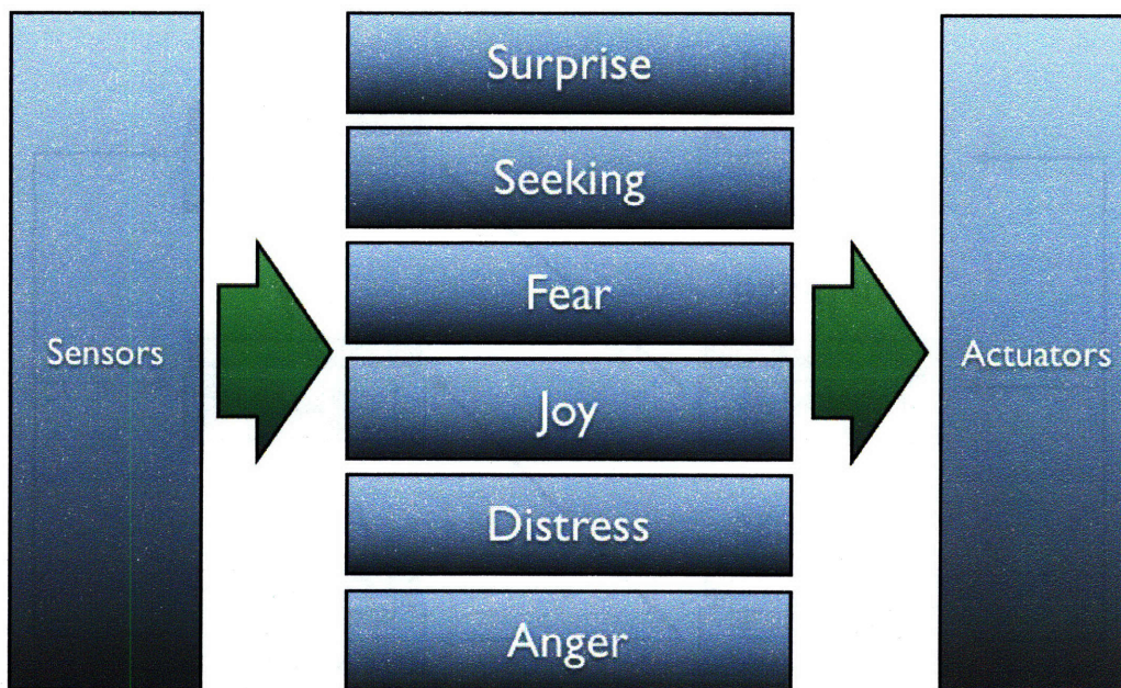
Figure 6-5: Affect Programs as systems in the Cathexis framework. This figure illustrates a more appropriate system-level view of the Cathexis framework. In this type of decomposition, all Affect Programs are seen as systems that receive information and influence behavior. Each of these systems has full access to all of the robot’s sensors and actuators. Despite the vertical organization of the figure, no hierarchy is implied, but the notion of parallel processing does apply: All systems have access to the same information and may process it simultaneously, but each system has its own processing style as described in the text.
