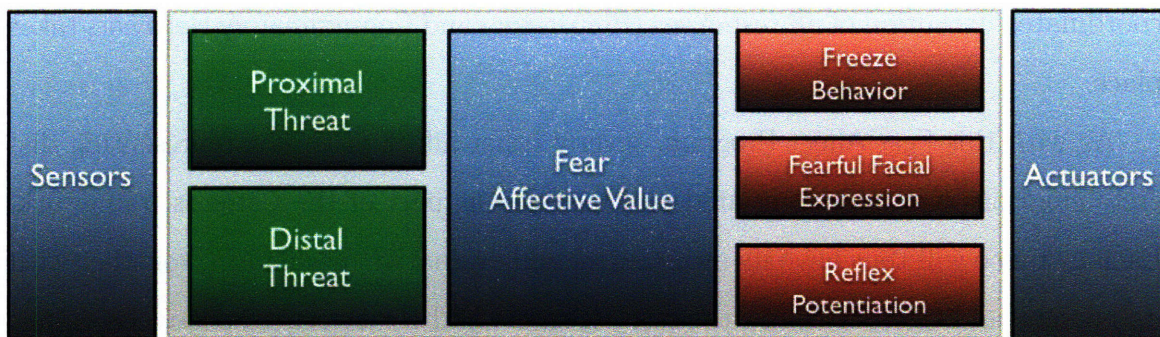
Figure 6-3: An instance of a Fear Affect Program. This figure illustrates a specific instance of the Affect Program abstraction. The Fear Affect Program showed here includes a set of Releasers that detect a threatening stimulus and determine the level of the threat depending on whether it is distal or proximal. The Fear Affective Evaluation Unit, depending on the significance of the stimuli would coordinate the associated behaviors, which in this case correspond to a Freezing Behavior, a Fearful Expression, and the internal mediation of mechanisms for Reflex Potentiation
