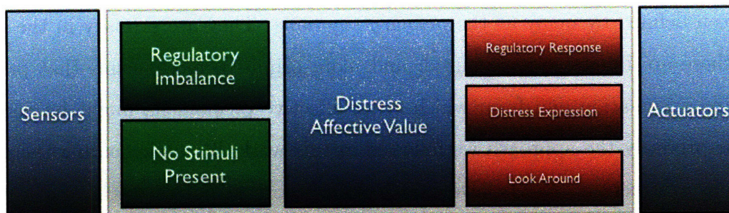
Figure 7-14: Illustration of an instance of the Distress Affect Program in the robot Yuppy. Three different pathways are coordinated by the Distress Affective Evaluation and Control Unit. The first pathway regulates seeking behaviors in search of objects of interest. The second pathway regulates sorrowful expressions according to the activity level of the Distress Affect Program. Finally, the third pathway mediates control responses that help the robot maintain balance of its regulatory mechanisms.
