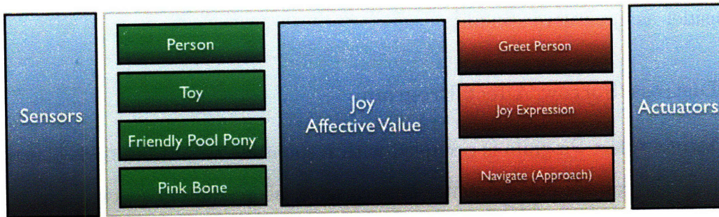
Figure 7-13: Illustration of an instance of the Joy Affect Program in the robot Yuppy. Three different pathways are coordinated by the Joy Affective Evaluation Unit. The first pathway regulates interactions with people through a Greet-Person Response. The second pathway regulates joyful expressions given the presence of any or all of the aforementioned stimuli. Finally, the third pathway mediates approach responses toward stimuli that were deemed “interesting” (see text).
