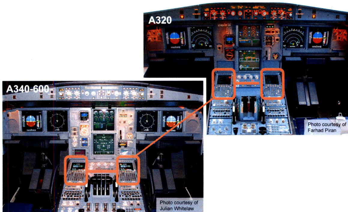
Figure IV-1: Pairs of MCDU units in the Airbus A320 & A340-600 models.
