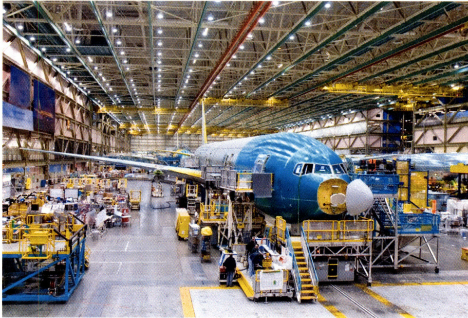
Figure VI-8: Moving assembly line of the Boeing 737NG sub-family at Renton 4 .
