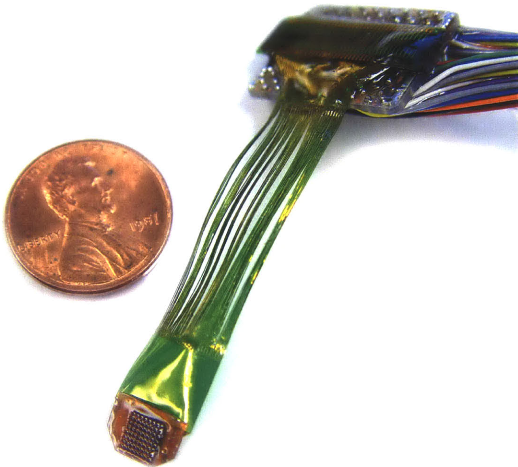
Figure 4-5. Image of an assembled TEAS microelectrode array assembly [11].
