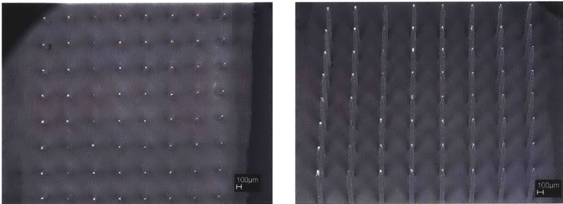
Figure 4-28. SEM images of a parylene-coated assembly, consisting of platinum-coated electrodes epoxied into a polyimide substrate, after the electrode tips have undergone laser ablation.
