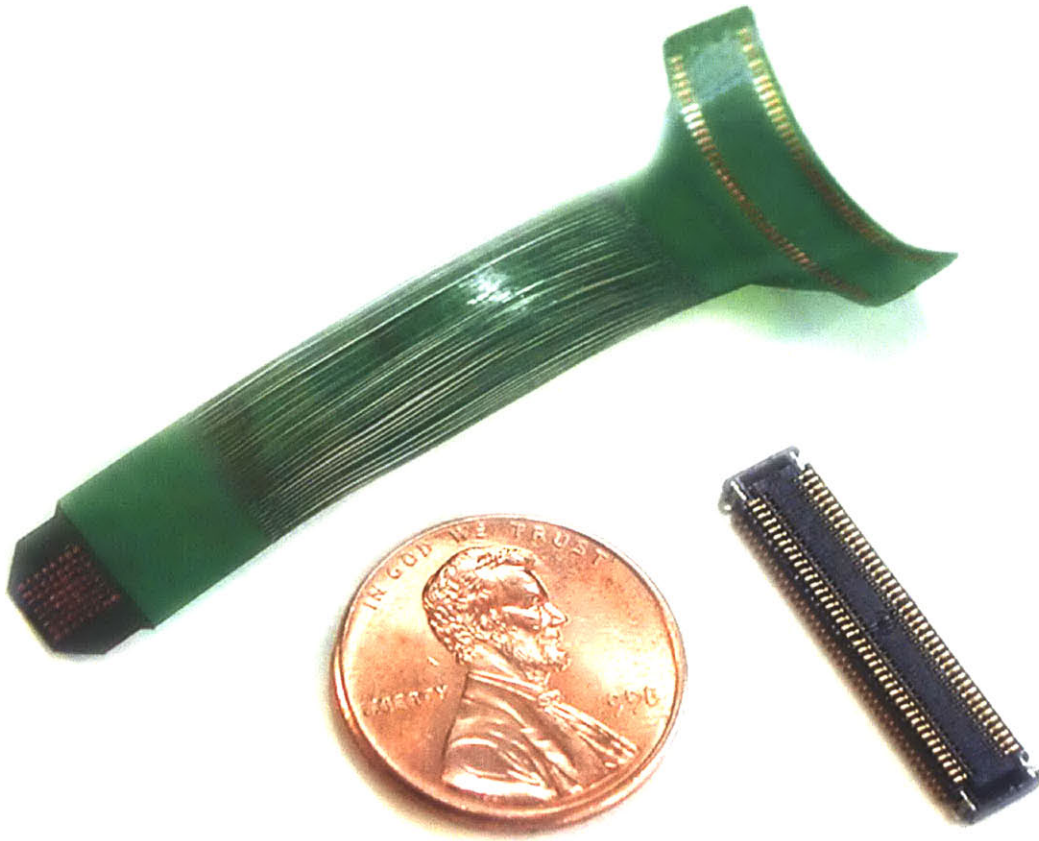
Figure 4-30. Image of the components of the TEAS prototype connector cable. They include a flexible PCB and an 80-pin connector [8,11]. (Photo: Jan Malášek)
