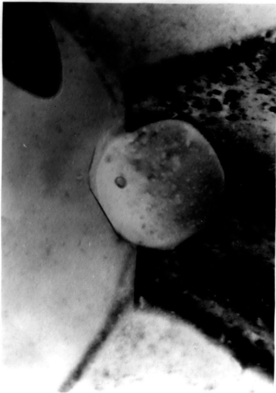
Figure 26. TEM micrograph showing oxide particle at grain boundary of alloy N-5.
