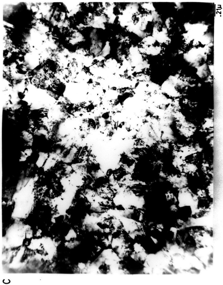
FIGURE 8. C. TEM MICROGRAPH OF ALLOY N-3 SHOWING HIGHLY WORKED STRUCTURE.
