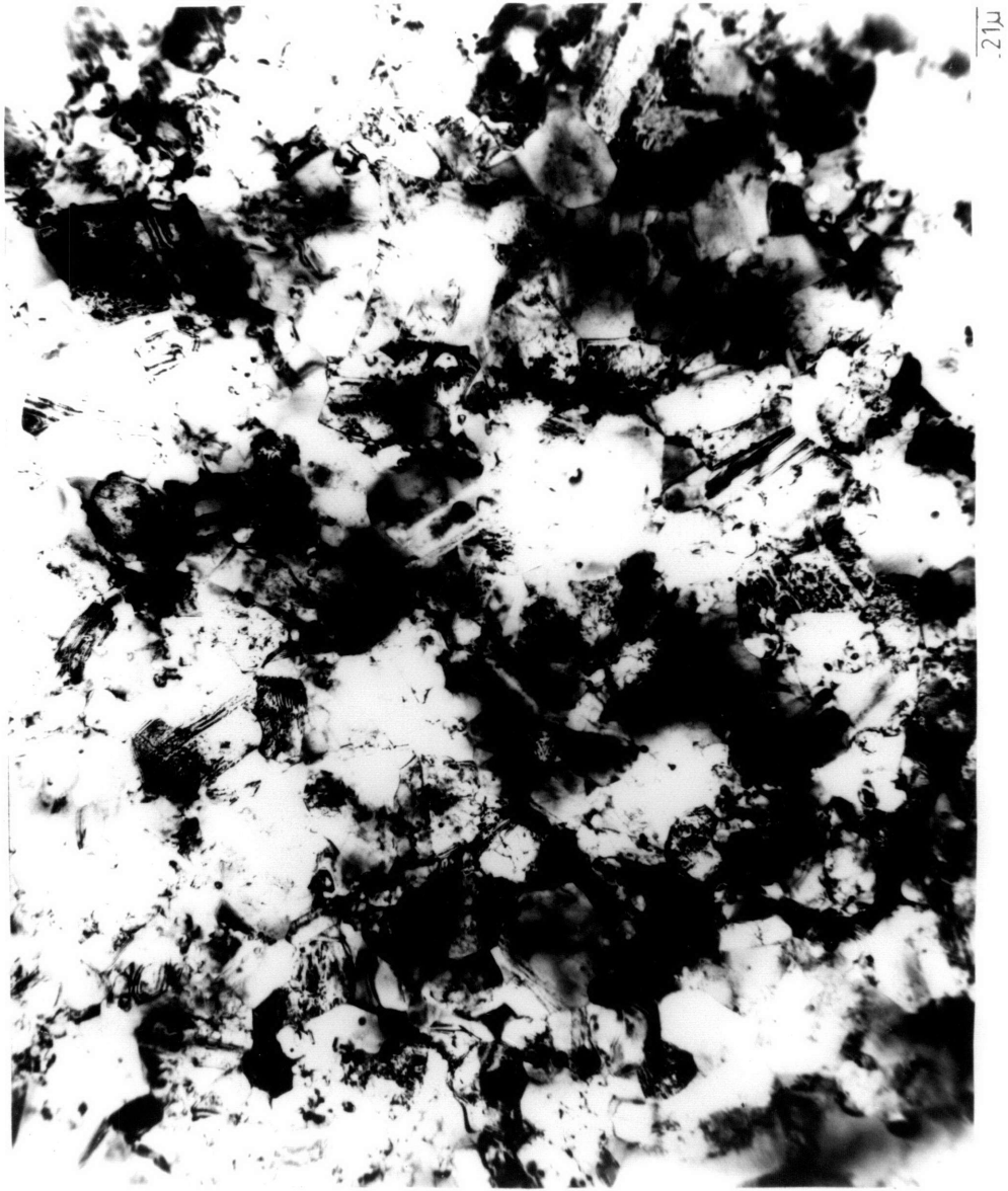
FIGURE 7. C. TEM MICROGRAPHS OF ALLOY N-2 SHOWING HIGHLY WORKED STRUCTURE.
