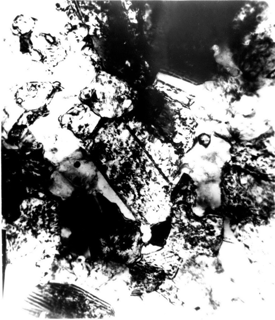
FIGURE 10. B. TEM MICROGRAPH OF AS-EXTRUDED N-5 SHOWING CELL FORMATION.
