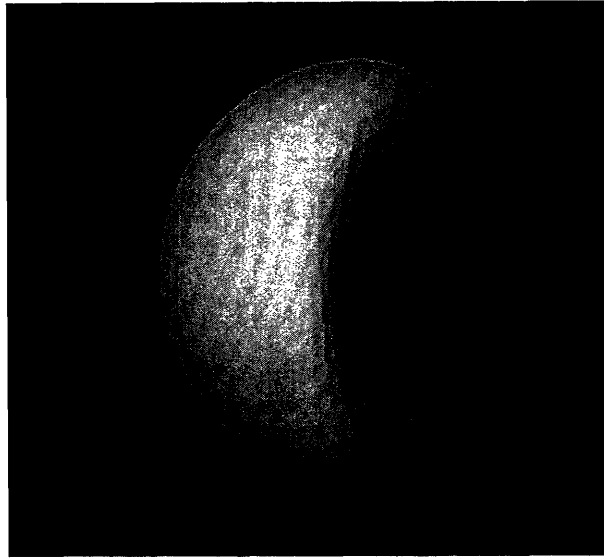
Figure 6-10. Haptic rendering of a deformable object. The small dark dot in the figure represents the probe. The original shape of the object is like a sphere. When the probe penetrates the surface of the object, the vertices of the object will be moved along the direction of penetration.
