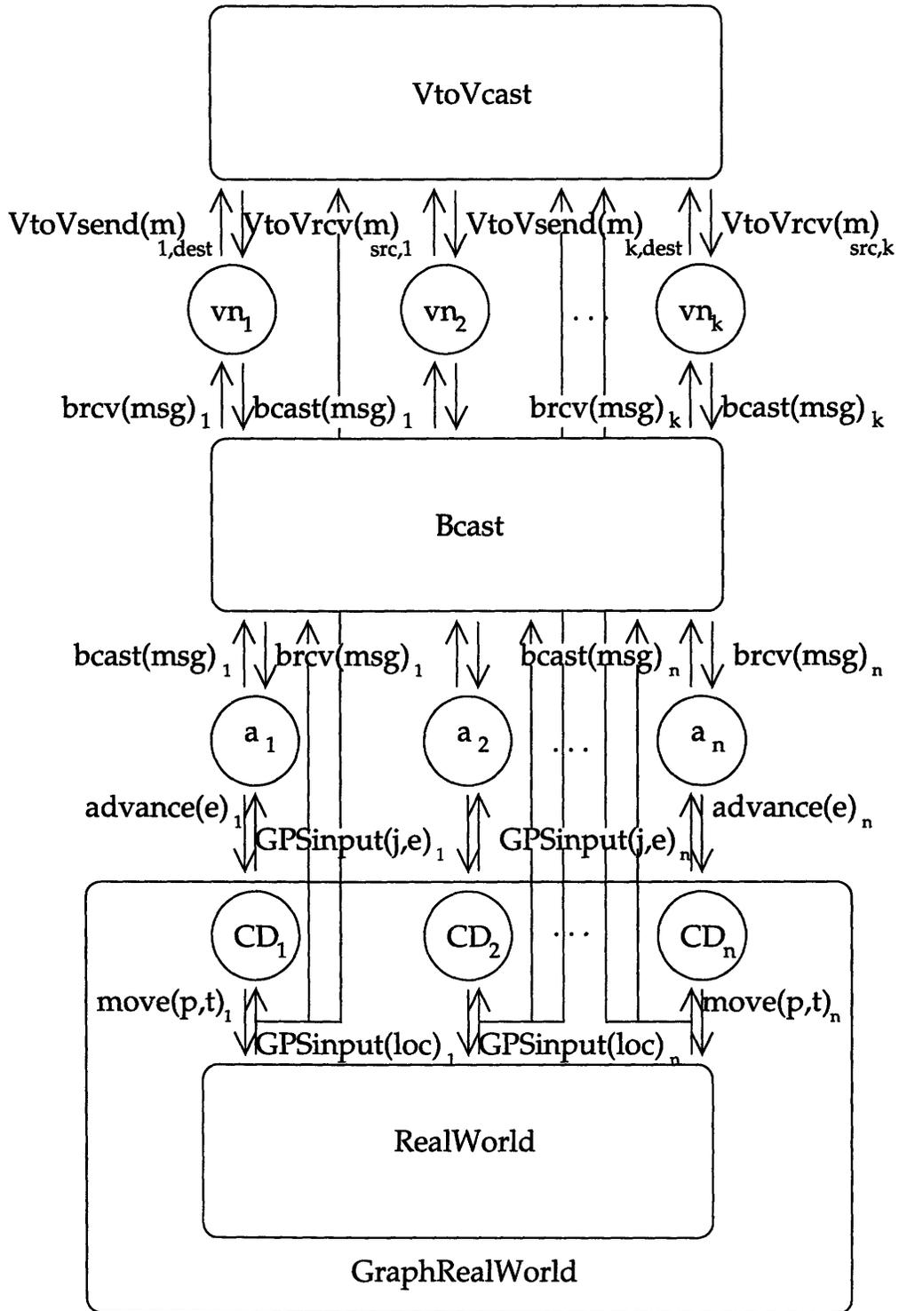
Figure 5-6: Emulation of the Known Path VSA Layer, for  $I = \{1, 2, \dots, n\}$ ,  $J = \{1, 2, \dots, k\}$
