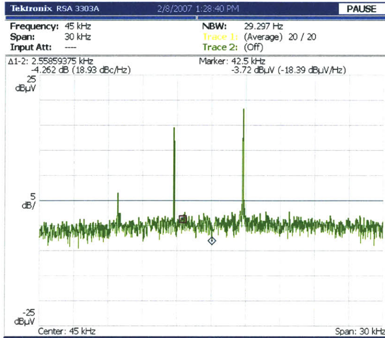
Figure 3-30: Voltage spectral density surrounding the carrier frequency of 42 kHz at the differential output of the front-end amplifier with no input signal and the inputs open-circuited. Interference from other lamps appear as stray signals in the plot.
