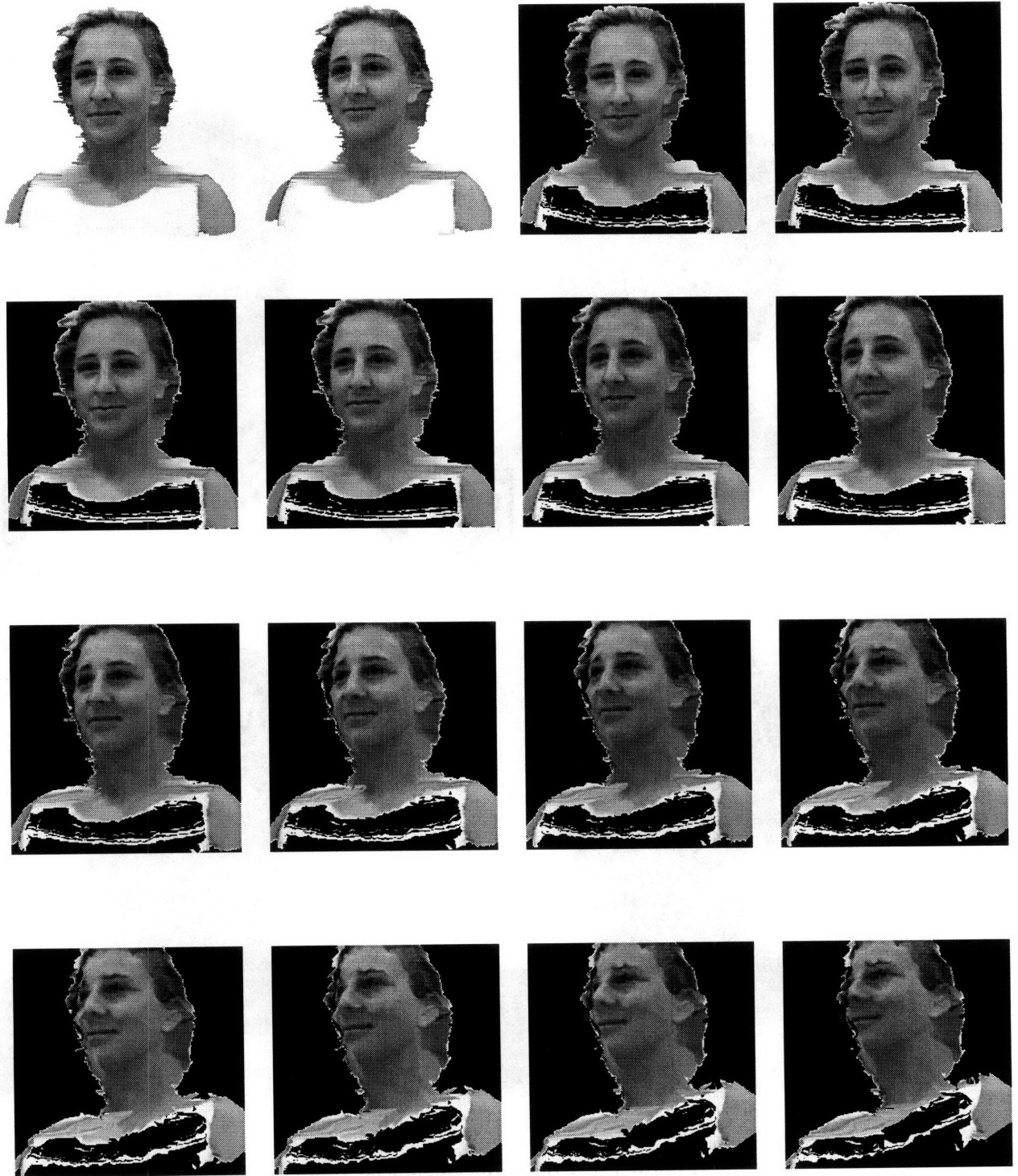
Figure 4-7: Movie 1: Both vertical and horizontal rotation of 3 degrees between consecutive images. The only real images are the first two ones on the left top.
