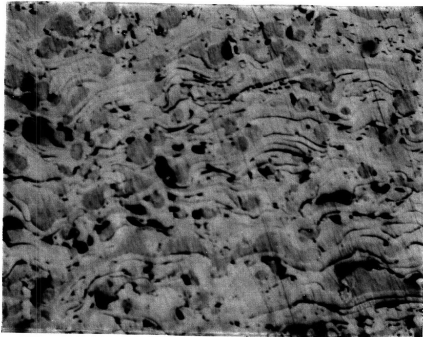
Figure 51. Different types of porosities found in the LDC deposit: (A) Solidification shrinkage, [X165] (B) crevices between splats, [X82.5] and (C) gas porosities, [X165] and [X1,800]
