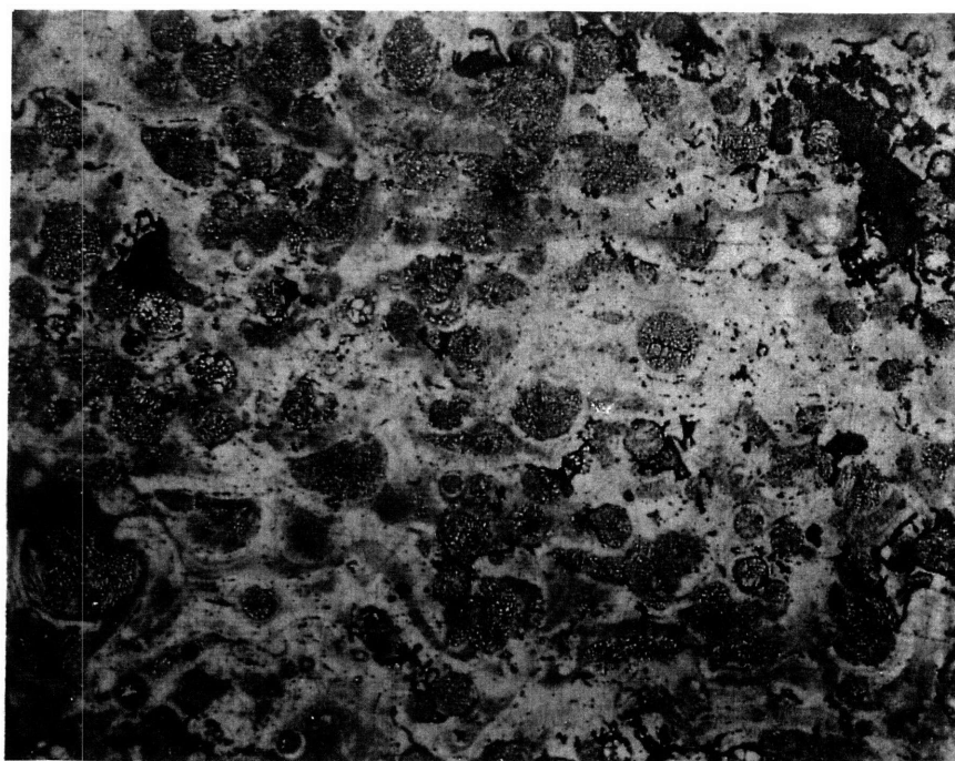
Figure 47. Agglomerates of unacceptable powder deposited by the spray back-tail at the bottom of run #78, which result from a wrong combination of process parameters.
