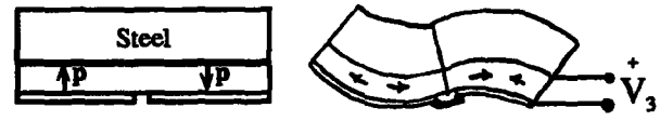
Figure 4: Neighboring electroded segments if alternately poled will strain oppositely when driven with a common voltage.
