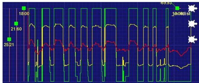
**Figure 4-32:** a graph showing how variables are mixed and the resulting output. Red (in the center) is the pendulum angle, green (the large blocky line) is the distance to the predicted position, yellow (in between the first two) is the average used to control the motor power.
