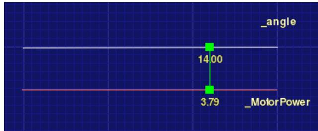
**Figure 4-25: Greg and Joe’s program using the line objects to convert the pendulum’s angle to control the car’s speed. The top line measured the pendulum’s angle. Its value was mapped to the line under it, which was used to control the motor power on the car.**
