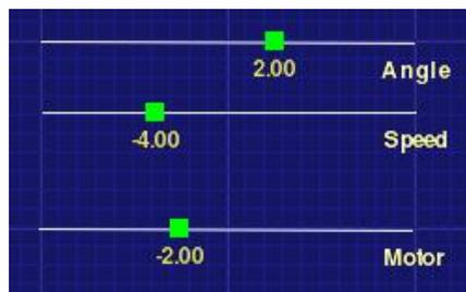
A similar program using the continuous method. The motor output power is the sum of Angle and Speed parameters
