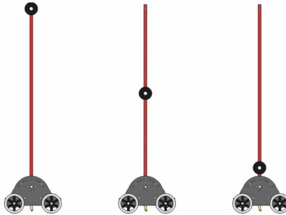
**Figure 4-8:** Albert and Anderson experimented to determine the optimum location for the stabilizing weight. The figure, from left to right, shows three locations that were tested: top, middle, and bottom. They then made recordings of the motions when being manually balance using their hand.
