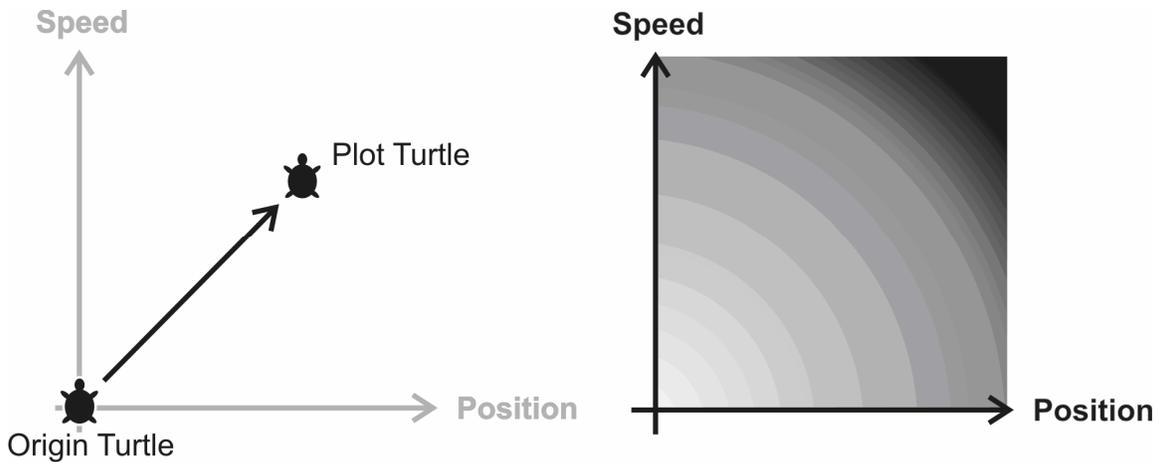
Figure 4-15: (Left) a turtle is placed at the graph's origin as a reference point. Plot turtle's location on the graph depends on the position and speed values. The distance between the two turtles is a vector with a length that determines the motor power. (Right) a color coded graph showing the motor power at each position/speed combination. The darker color means higher motor power.
