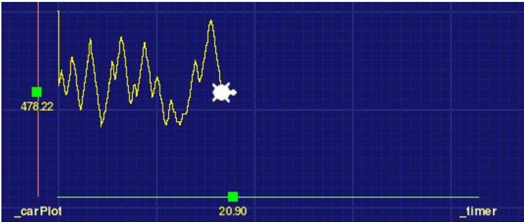
Figure 6-8: An example of a simple graph. The `_carPlot` line is the car position value while the `_timer` line is an auto increment counter line. The turtle position is the (X,Y) combination of the value positions on the screen.
