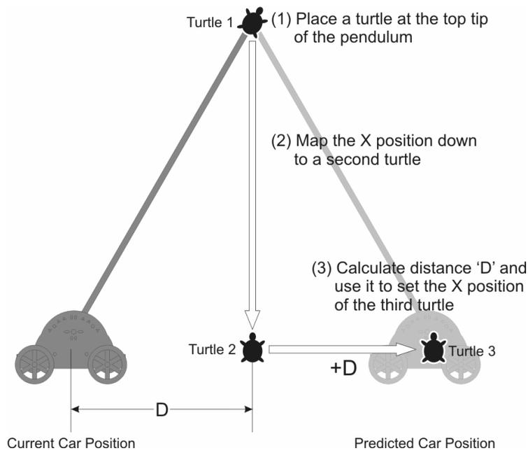
**Figure 5-2: The operations performed by Greg to figure out where the car should move to given the starting position.**
