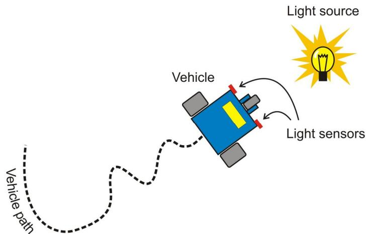
**Figure 3-2: Another situation where thinking locally can yield a global behavior. The vehicle appears to move towards the light. This behavior is exhibited by telling the robot to repeat “turn a little towards the brighter side and move forward a little.”**
