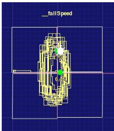
**Figure 4-40: The ring.** A ring shape was observed when the system stays in control. A large ring indicates large vibrations.
