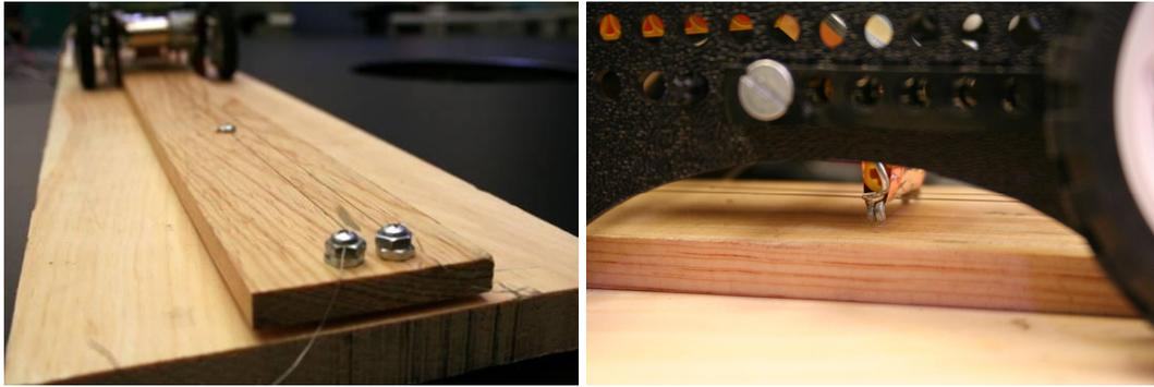
**Figure 3-6:** The position of the pendulum car was sensed using a pair of Nichrome wires, which was strung across the length of the wood platform (left). The car has a small conductive stub (right) connecting the wire at the car's current position.
