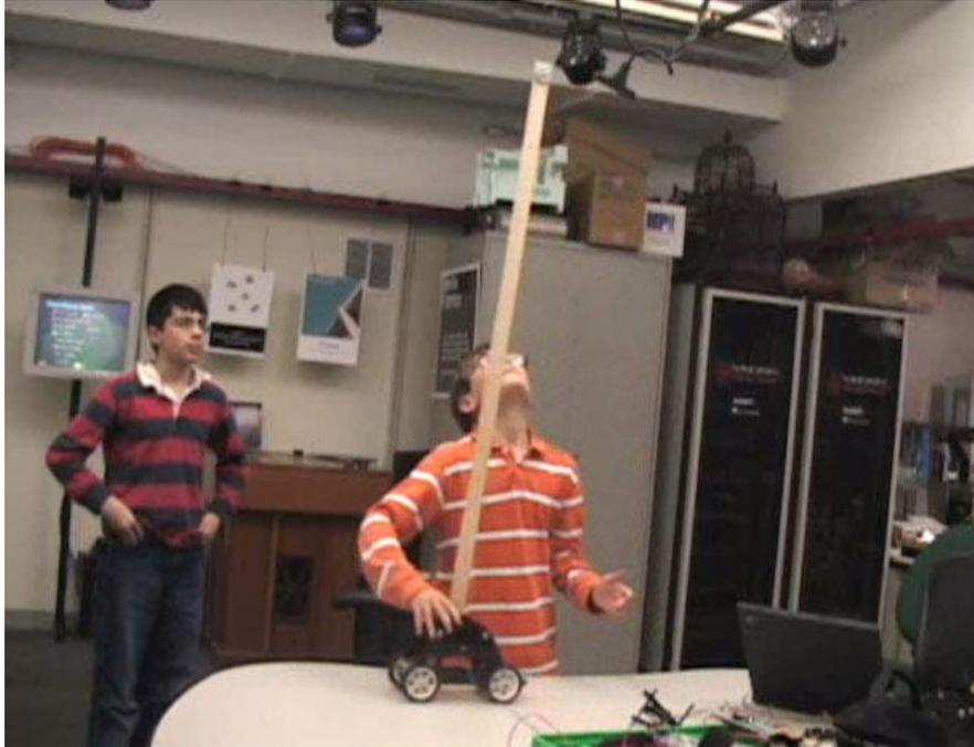
**Figure 3-3: Students playing with the inverted pendulum. The pendulum is connected to a car at the base. This restricts (and simplifies) the controlling gesture to a one-dimensional motion on a linear path.**
