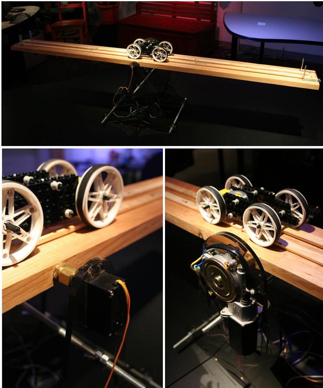
**Figure 3-9:** Photo of the balance beam (top), a servo motor hacked to function as an angular sensor (lower left), and the driving 12V DC motor (lower right)
