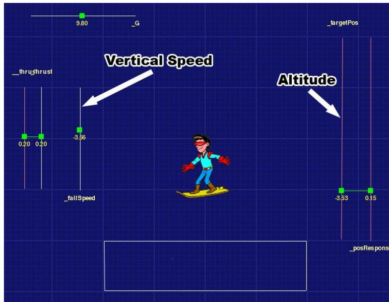
Figure 4-35: An overview of the hover board simulation. The main character on the board is pulled downwards by gravity. The board can thrust either towards or away from the ground. The board's altitude and vertical speed are provided through the vertical lines.
