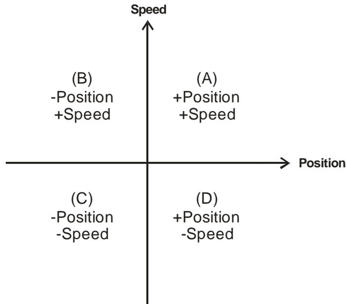
**Figure 4-14: An illustration of the four states that represents the possible combinations of the position and speed variables.**
