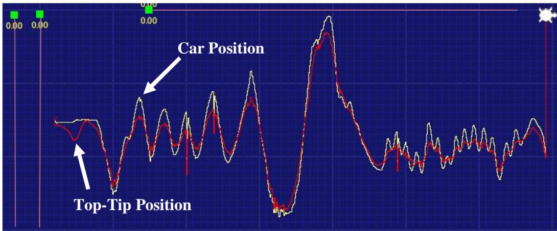
**Figure 4-24:** An example of Joe's recording. The red line represents the motion of the top tip and the yellow line shows the motion of the car. The recording was made while Joe was balancing the pendulum-car with his hand. Joe was trying to use graphs like this to prove that rapid motion of the base (right half of the graph) yields less motion of the top tip than trying to keep the beam still (left side of the graph).
