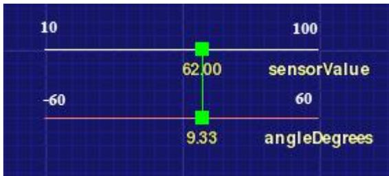
Figure 6-1: An example of how line objects can be used to scale and convert values
