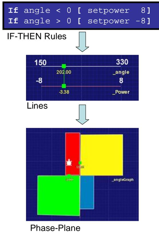
**Figure 5-1:** The representation of state evolved from simple IF-THEN rules (top) to the researcher’s Lines approach (middle). The Phase-Plane controller (bottom) was a result of the researcher’s observation of the students’ thinking combined with the researcher’s knowledge about what is needed.
