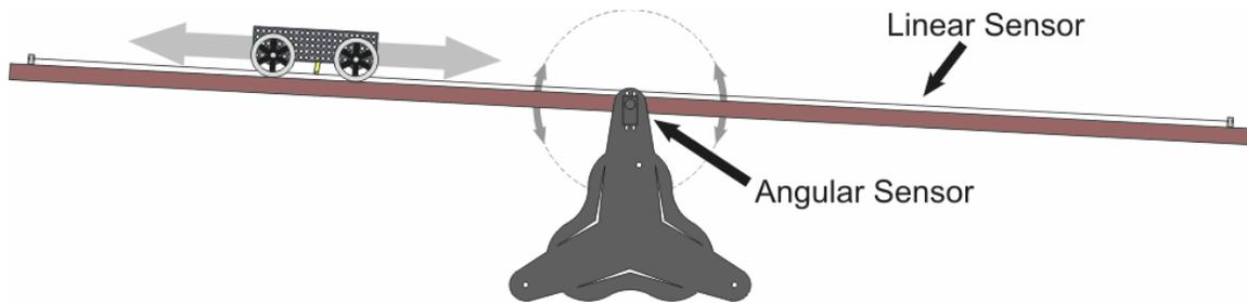
**Figure 3-8: Construction of the balance beam task**
