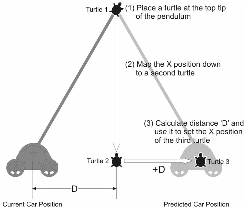
**Figure 4-29: The three step process used to approximate the position to which the pendulum car should move.**
