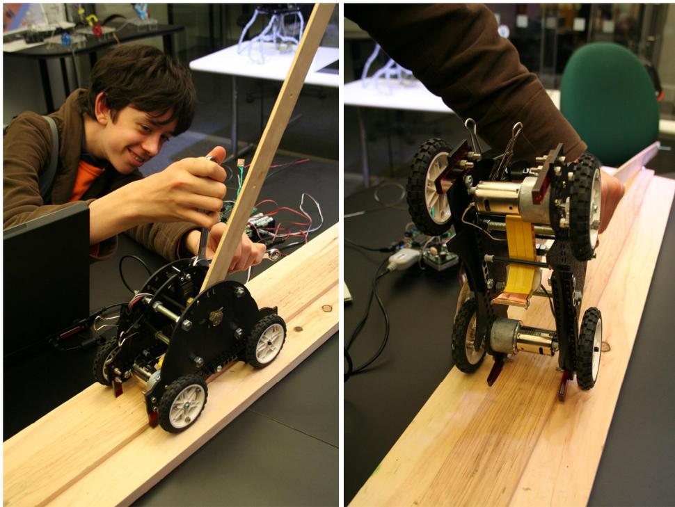
**Figure 3-7:** The pendulum car shown from the top (left) and from underneath (right)
