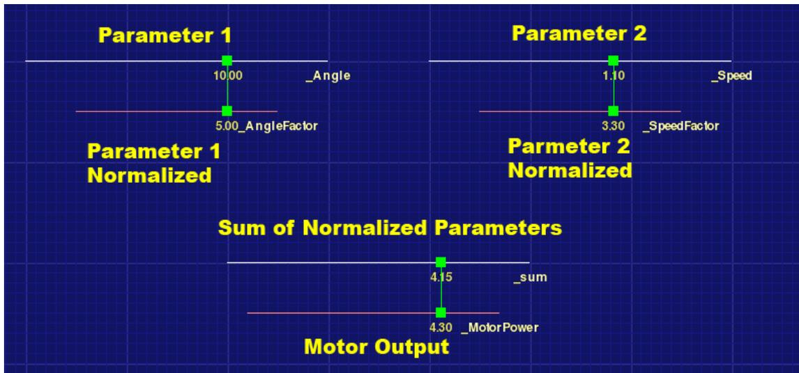
**Figure 4-26:** The initial program that used both the pendulum’s angle and the tip speed to control the car. Both the input parameters (`_Angle` and `_Speed`) were normalized (`_AngleFactor` and `_SpeedFactor`) and summed together (`_sum`). The sum was then used to produce the motor power that drives the car.
