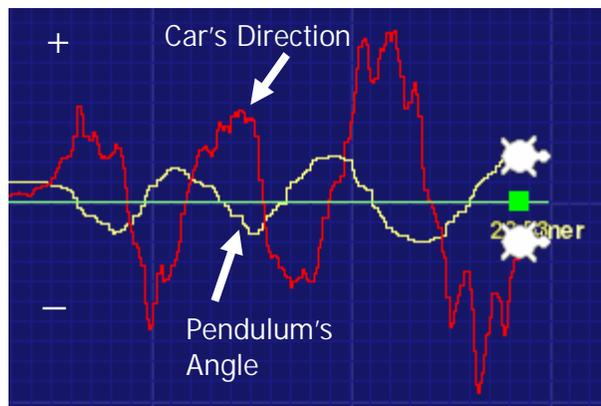
**Figure 4-6:** An example of a graph that was created to analyze the car’s direction and the pendulum’s angle. If the car were to always follow the pendulum’s angle (as Albert and Anderson thought), both lines would always be on the same positive or negative halves (above or below the center horizontal line). The graph clearly shows that this is not the case. The car speed and pendulum’s angle are often in opposition.
