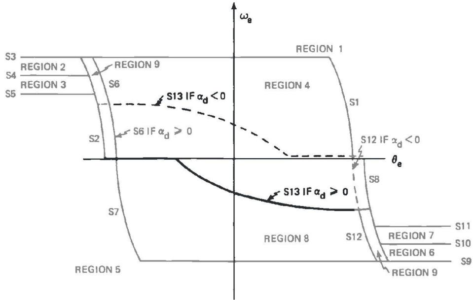
**Figure 4-18: A Phase-Plane diagram used to implement the shuttle's RCS system. Different regions were defined to tell the craft what state it was in. Switch lines (S13) were used to determine when to fire the appropriate thrusters when the shuttle was in regions 4 and 8.**
