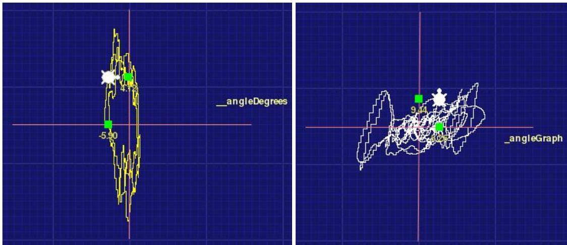
**Figure 4-13: A comparison between an inverted pendulum controlled by the hand (left) versus one that was controlled by the student’s program (right). The rectangles that defined the states were removed from the figures for the clarity of the lines.**
