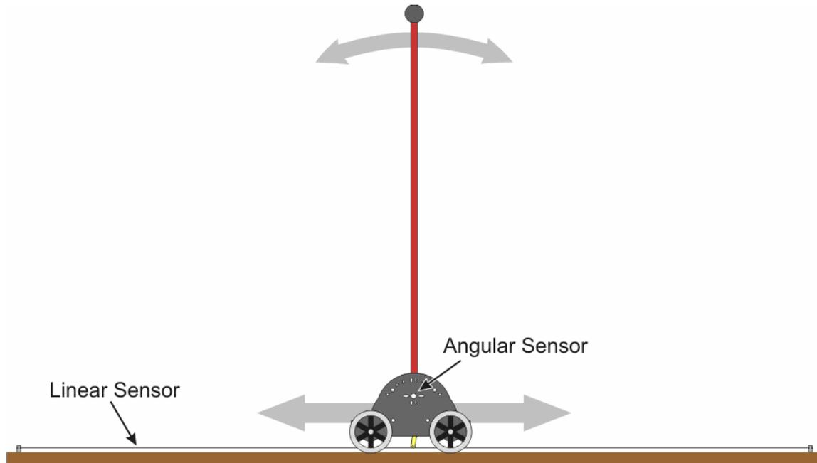
Figure 3-5: Construction of the inverted pendulum task
