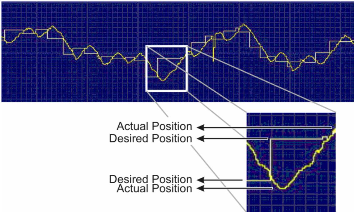
**Figure 4-30:** A graph showing the desired (predicted) position versus the actual car position. The blocky line shows the desired car position calculated by the prediction system while the curvy line shows the actual car trajectory. It can be seen that the car always exceeds the desired position causing what Greg has identified as an overshooting problem.
