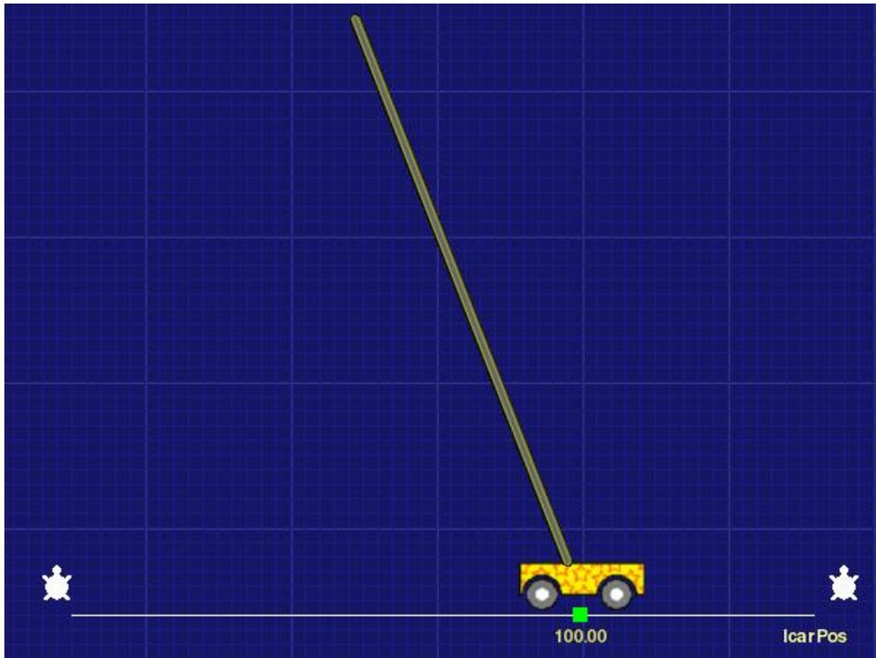
**Figure 6-11: Screen shot of how two turtles are placed at each side of the screen to stop the car from falling off the table.**
