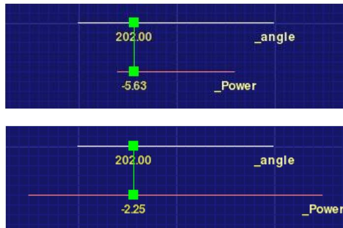
**Figure 4-3: The conversion between two line objects can be influenced by changing the line’s length. The upper figure shows how a shorter `_power` line increases the power value in response to the angle. An angle value of 202 is converted to a power of -5.63. The lower figure shows the opposite when the `_power` line is expanded. An angle value of 202 is now converted to a power of -2.25.**
