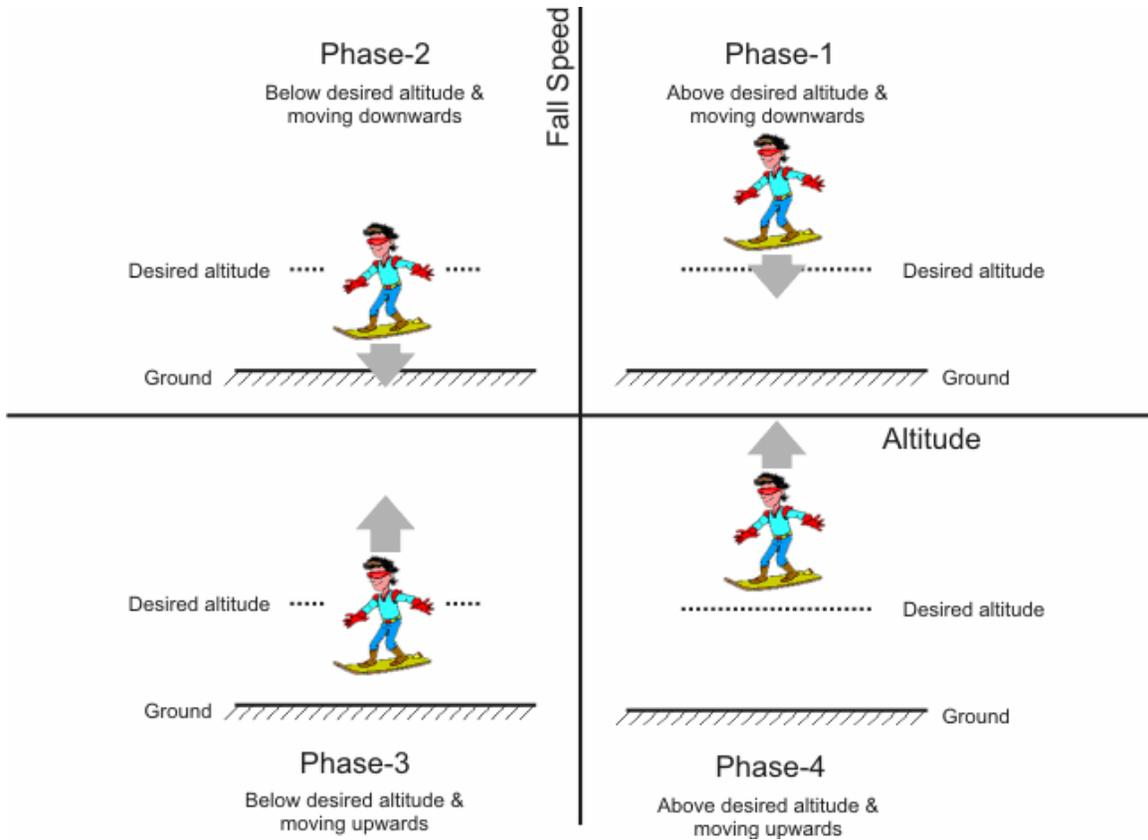
**Figure 4-37: A graphical illustration of the four phases, which are the mix of two variables: Altitude and fall-speed.**
