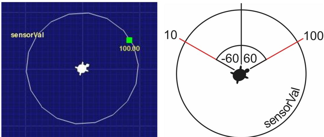
**Figure 6-2: Another method to convert sensor data to an angle value by using a circle line and a turtle. (Left) a screen shot of the process in action. (Right) a diagram showing the needed alignments to make the conversion work.**
