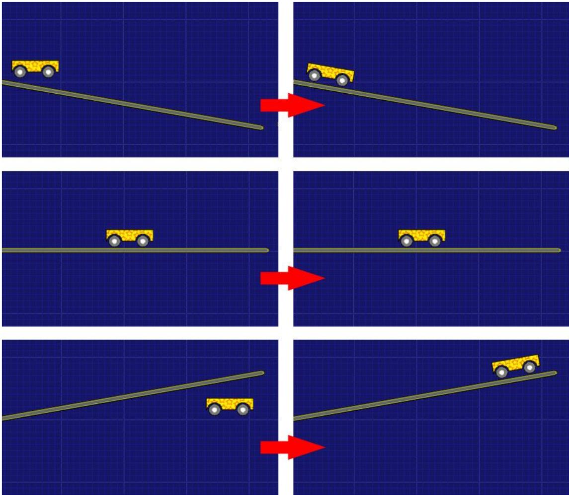
Figure 6-6: The left column shows the car’s linear movement with no relationship with the beam. The right column shows the same car motion after establishing a “stickto” relationship with the beam.
