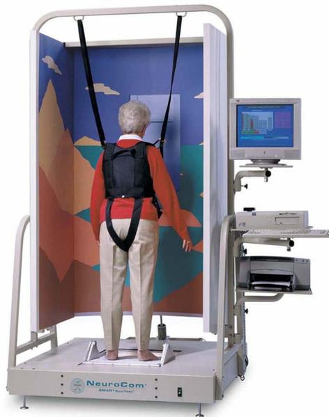
**Figure 2-1: An example of CDP data collection device. Human gait control under various perturbations is recorded through electronic sensors for later analysis.**
