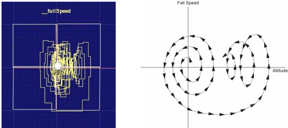
**Figure 4-39: The Helix.** The graph shows the trail after phase-1 (the upper right box) was fixed. The system behaved better but still produces occasional disruptions due to the remaining problem in phase-3, which still unnecessarily fires the thrusters. A helix was observed when the system was gradually recovering from the disruption.
