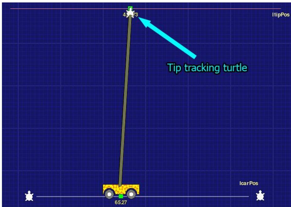
**Figure 4-9:** showing how the pendulum’s top tip was determined by sticking a turtle to the on-screen pendulum object. The tracking turtle’s X coordinate is the desired position.
