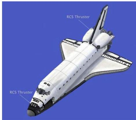
**Figure 4-17: The space shuttle's on-orbit reaction control system (RCS) utilizes multiple thrusters distributed throughout the head and tail sections.**
