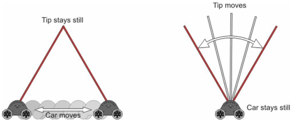
**Figure 4-23: Two reference points. The tip can be seen as the part that tends to move the least in relation to the environment (left) or it can be seen as the part the moves the most in reference to the car (right)**
