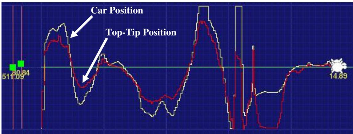
**Figure 4-10:** Graphs showing movements of the pendulum's top tip (red) and the car (yellow). The car was manually controlled by the hand. The top, middle, and bottom graphs show movements when weights are attached to the top, middle, and bottom respectively. Weight at the top tip has noticeably less movement.
