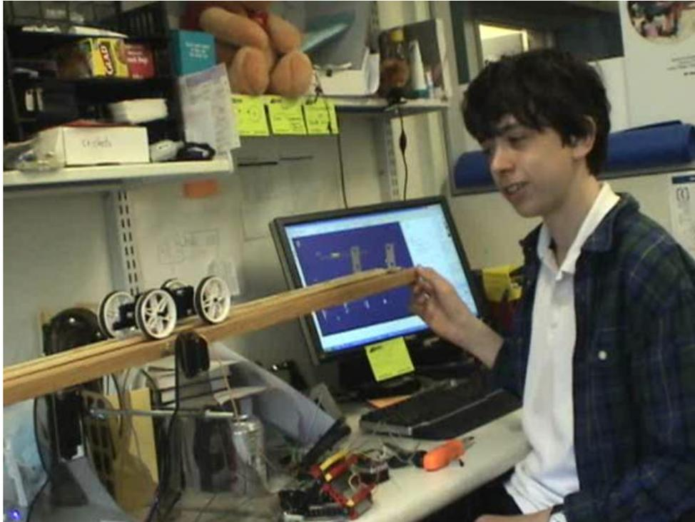
**Figure 3-4: The balance beam as it is being manipulated by a student. The goal of this challenge is to prevent the rolling car from falling off the beam.**
