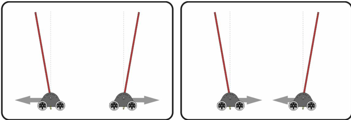
**Figure 4-5:** The left box shows the rules that are present in Albert and Anderson’s program. That is, the car should always move in the direction of the pendulum’s angle. The right box shows new states that were observed in the recording of hand balanced sessions where the car was seen to move in the opposite direction of the pendulum’s angle.
