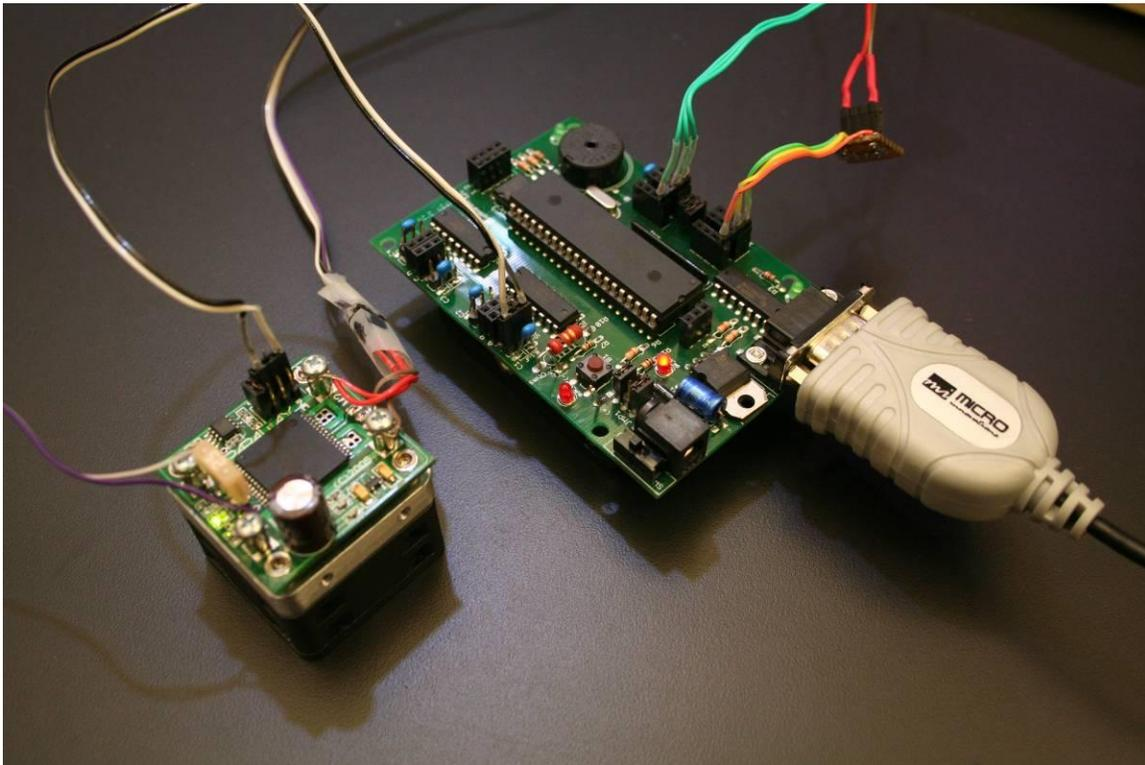
**Figure 3-10: The GoGo Board (right) was used to connect the sensors to the computer. It also controlled the motor driver unit (left), which took care of the torque and spin direction of the motor.**
