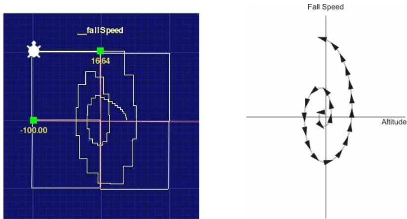
**Figure 4-38: The Spiral.** The outward spiral was caused by Greg's buggy program. The system failed to maintain stability.
