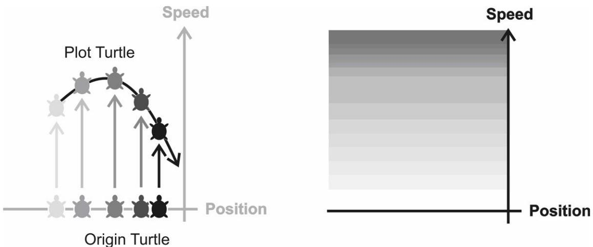
Figure 4-16: (left) to eliminate the motor jerks caused during state transitions, the position variable was removed from the distance vector in state B and D. This was accomplished by vertically aligning the origin and plot turtles. (Right) a color coded graph showing the motor power at each position/speed combination. The darker color means higher motor power.
