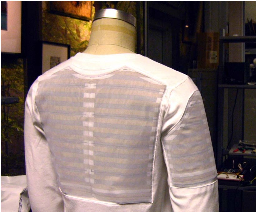
Figure 10. QTC sensors on the back and upper arm of the Wearable Witness .
