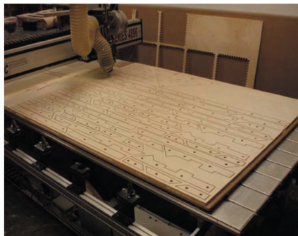
CNC Machine Cutting Layers
