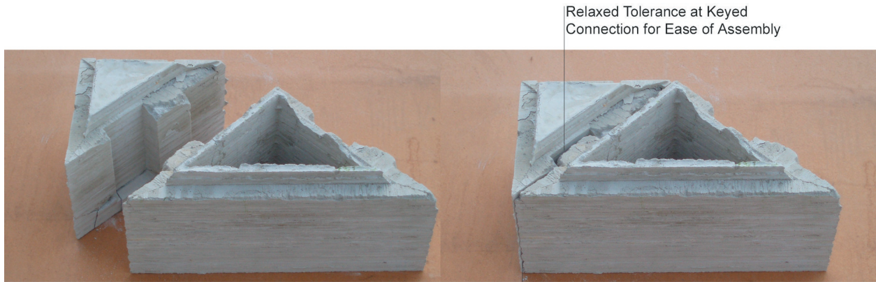
End Block & Full Mid Block
