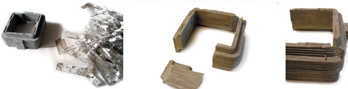
Cast Broken During Layer Removal
