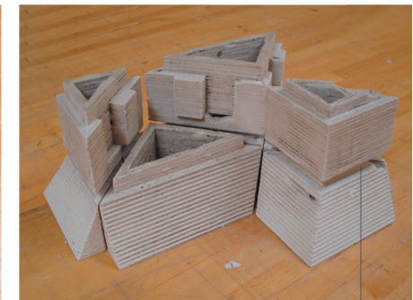
Units Did Not Slide Together as Anticipated
