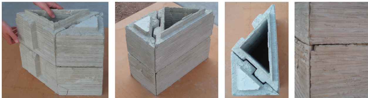
Full Scale Assembly - Horizontal & Vertical Connections
