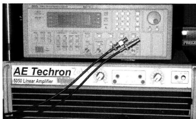
Figure 2-4: Waveform generator and Linear amplifier.
