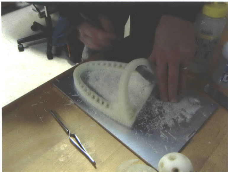
Figure 4.22 Rapid prototype model of the Chandelier wing section being manually excavated and cleaned.
