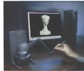
Figure 2.1 Chen, Sculpting system using the PHANTOM Desktop haptic interface.
