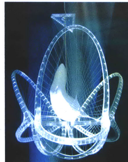
Figure 4.20 Early version of a physical prototype of the Chandelier constructed from laser-cut acrylic and plastic line. Digital templates, extracted from the Rhino 3D master model, were used by the laser cutter to precisely fabricate the curved pieces with exact spacing of the notches which hold the strings in position. Such precision is very difficult without a digital archetype.
