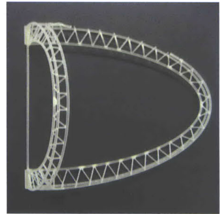
Figure 4.23 Excavated rapid prototype of the wing section.
