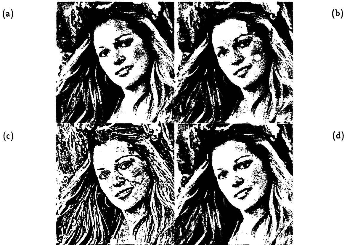
Figure 5.3: Performance of receiver-compatible system in the presence of interchannel interference (20 dB SNR): (a) Original picture. (b) NTSC encoding and decoding. (c) Receiver-compatible encoding and NTSC decoding. (d) Receiver-compatible encoding and decoding.
