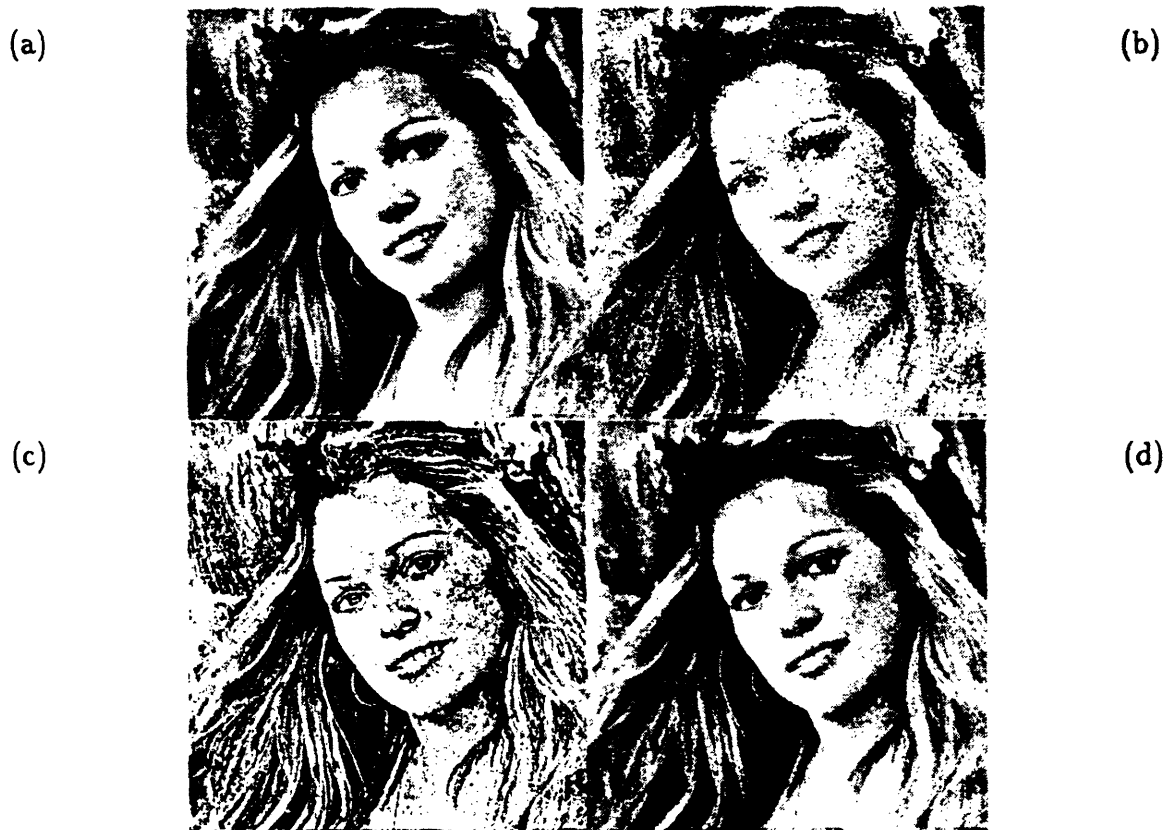
Figure 5.4: Performance of receiver-compatible system in the presence of additive random noise (20 dB SNR), multipath (20 dB SNR), and interchannel interference (20 dB SNR): (a) Original picture. (b) NTSC encoding and decoding. (c) Receiver-compatible encoding and NTSC decoding. (d) Receiver-compatible encoding and decoding.
