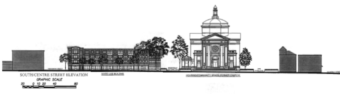
Figure 4. CSCP proposed re-development of the Blessed Sacrament Campus Centre Street elevation. The depiction has the rectory moved further down Creighton Street to allow for the larger mixed-use structure on the corner of Centre Street and Creighton Street.
