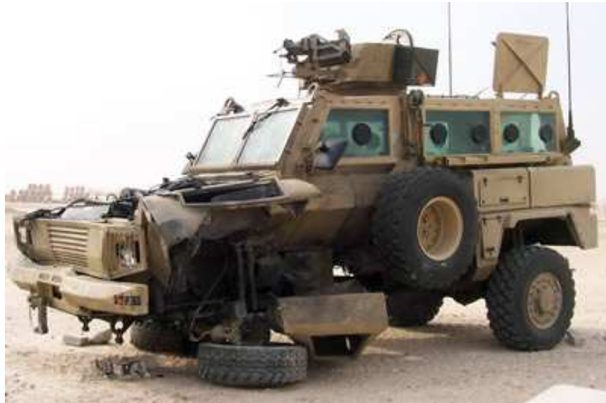
Figure 1-4: RG-31 vehicle after an attack with an improvised explosive device near Camp Taqaddum, Iraq [123].
