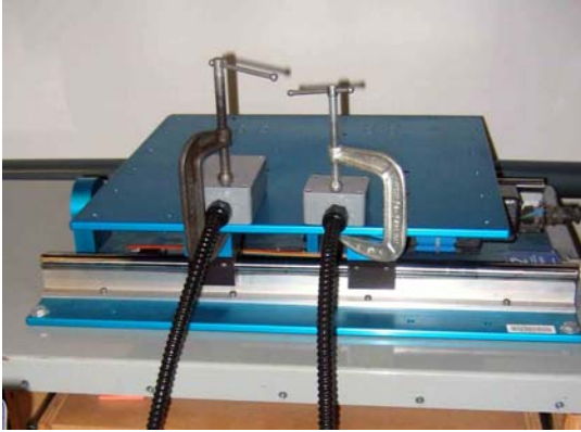
Figure 5-39: Horizontal shake device with two accelerometers attached.
