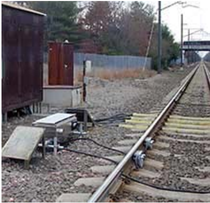
Figure 4-1: TBOGI laser sensor for misaligned bogie detection at Mansfield, MA (WID website).
