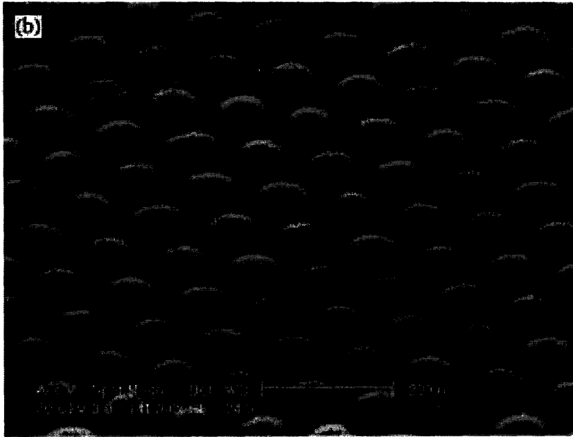
Figure 2.17: High magnification view of Ge nanodot array fabricated using alumina membrane. 37
