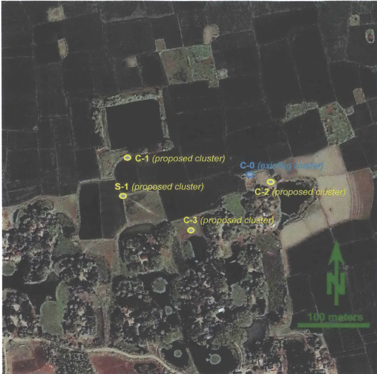
Fig.4.4 Secondary Well Clusters (C1, C2, C3 and S1): Based on the pond hypothesis, four new clusters of wells have been installed – three beside ponds, and away from the pond in the middle of the rice-field. According to the hypothesis (Fig.4.3), the arsenic concentration is assumed to be higher at shallow depths at the clusters C-1, C-2, and C-3, whereas the arsenic profile at cluster S-1 is thought to be somewhat similar to that of cluster C-0.
