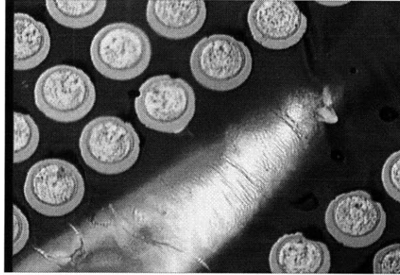
Figure 4-20: Semiconductor remain after InGaP etch, due to unetched GaAs during tier etch.
