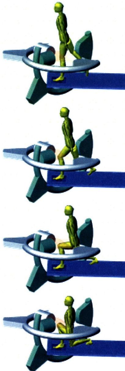
Fig. 4.1 Representation of single leg weight-bearing flexion of the knee while the dual-orthogonal fluoroscopic system captures the knee images.
