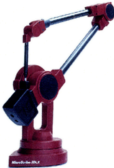
Fig. 8.3 The MicroScribe three-dimensional digitizer
