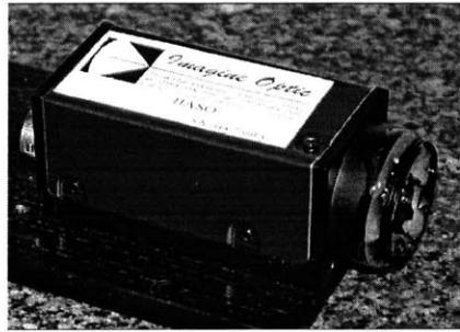
Fig 6.1. Shark-Hartmann wavefront sensor [8]
