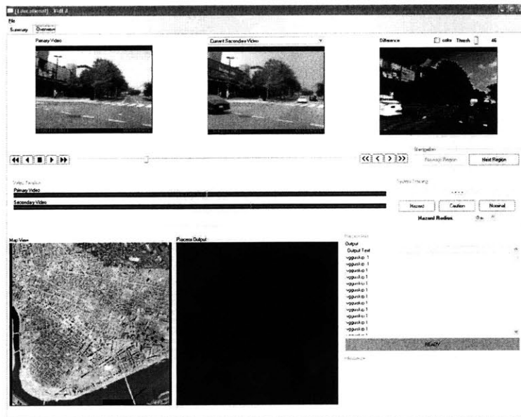
Figure 4-9: Screen-shot of the Overview tab in the Graphical User Interface. The synchronized views show a matching and corresponding difference image. The video time-lines show the positions of the displayed frames in the input video pair.
