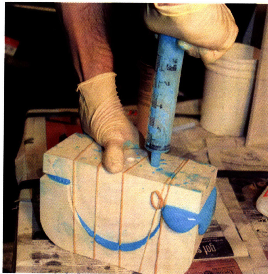
Figure 7-27: Injecting silicone into one mold set.
