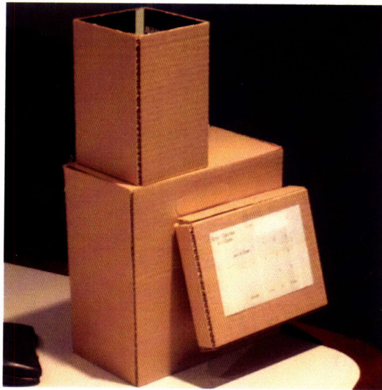
Figure 7-1: Early cardboard mockup of robot form.
