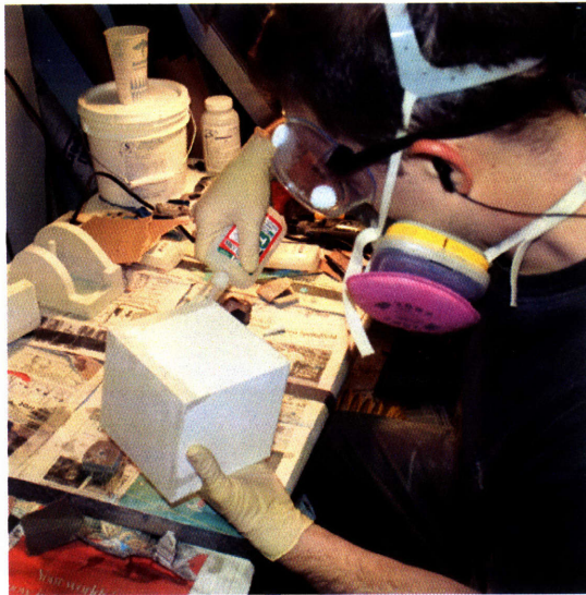
Figure 7-24: Applying cyanoacrylate to harden molds.
