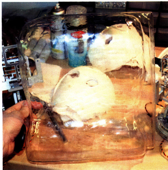
Figure 7-19: Thermoformed body shell before painting.
