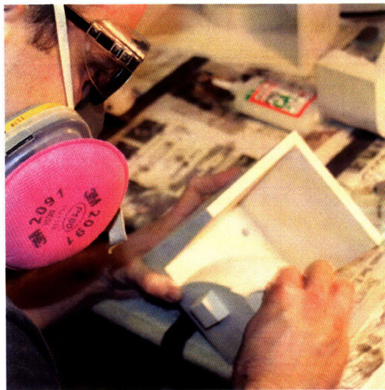
Figure 7-25: Sanding molds before using to make plastic parts
