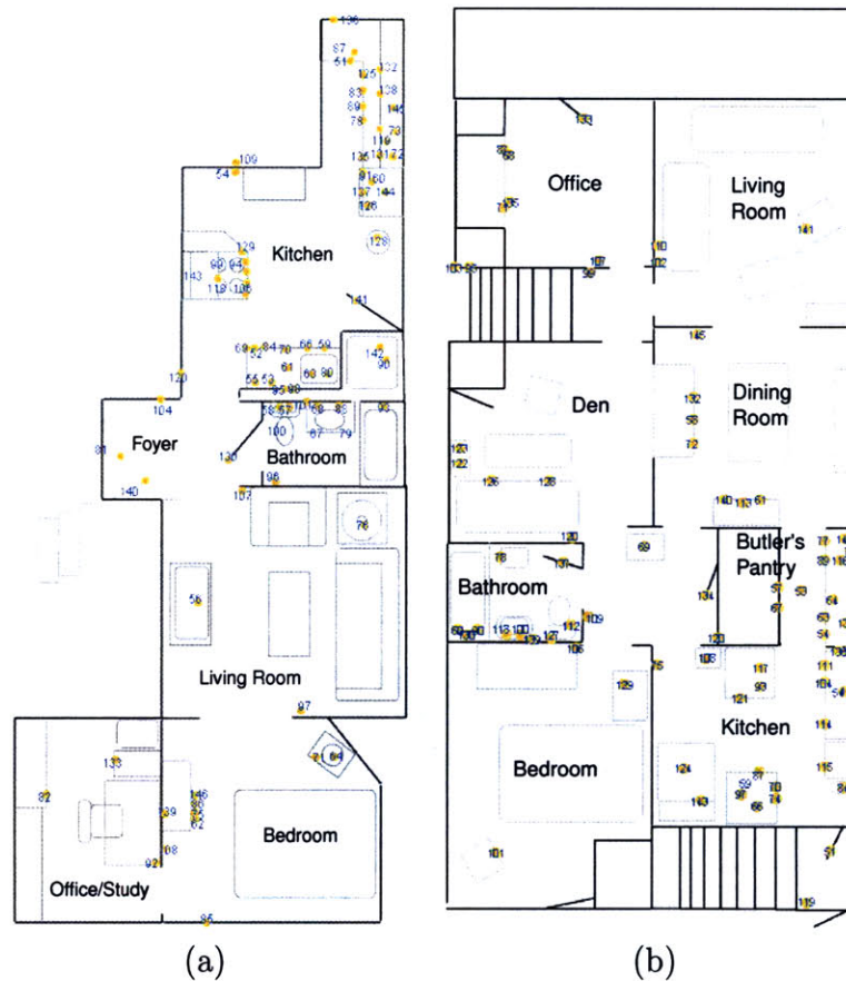
Figure 5-2: (a) The top view of the apartments and the sensors distribution for subject one. (b) Sensor distribution for subject two.
