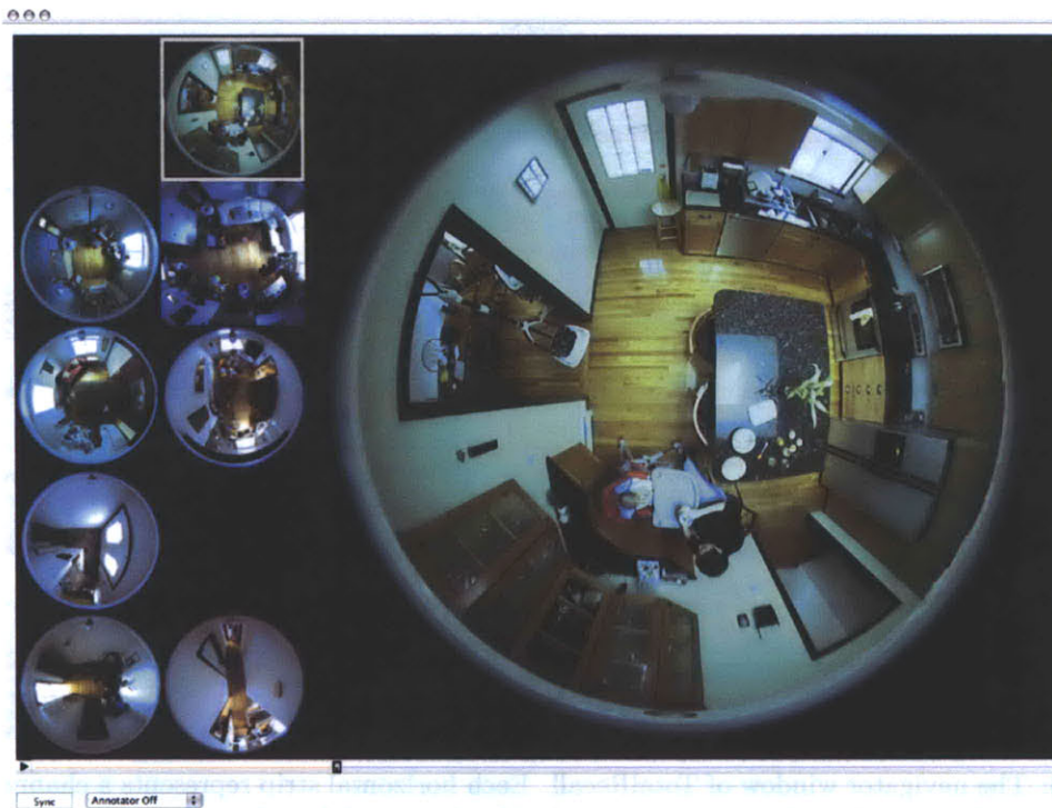
Figure 4.5: The TotalRecall video player displays ten channels of reduced resolution video and one channel of full resolution video. Video annotations may be entered directly onto the video (see 5).
