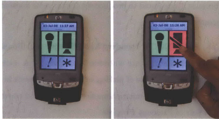
Figure 3.4: PDAs mounted in each room provide a control interface for the recording system. Each PDA has four buttons: (1) the top-left toggles audio recording throughout the house; (2) the top-right toggles video recording for one room; (3) the bottom-left button deletes a portion of recently recorded data to be deleted; and (4) the bottom-right can be pressed to mark events of interest.
