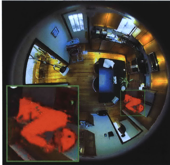
Figure 5.5: Pixel weights, indicated in red, are computed for each pixel in the bounding box based on color value frequencies and segmentation information.
