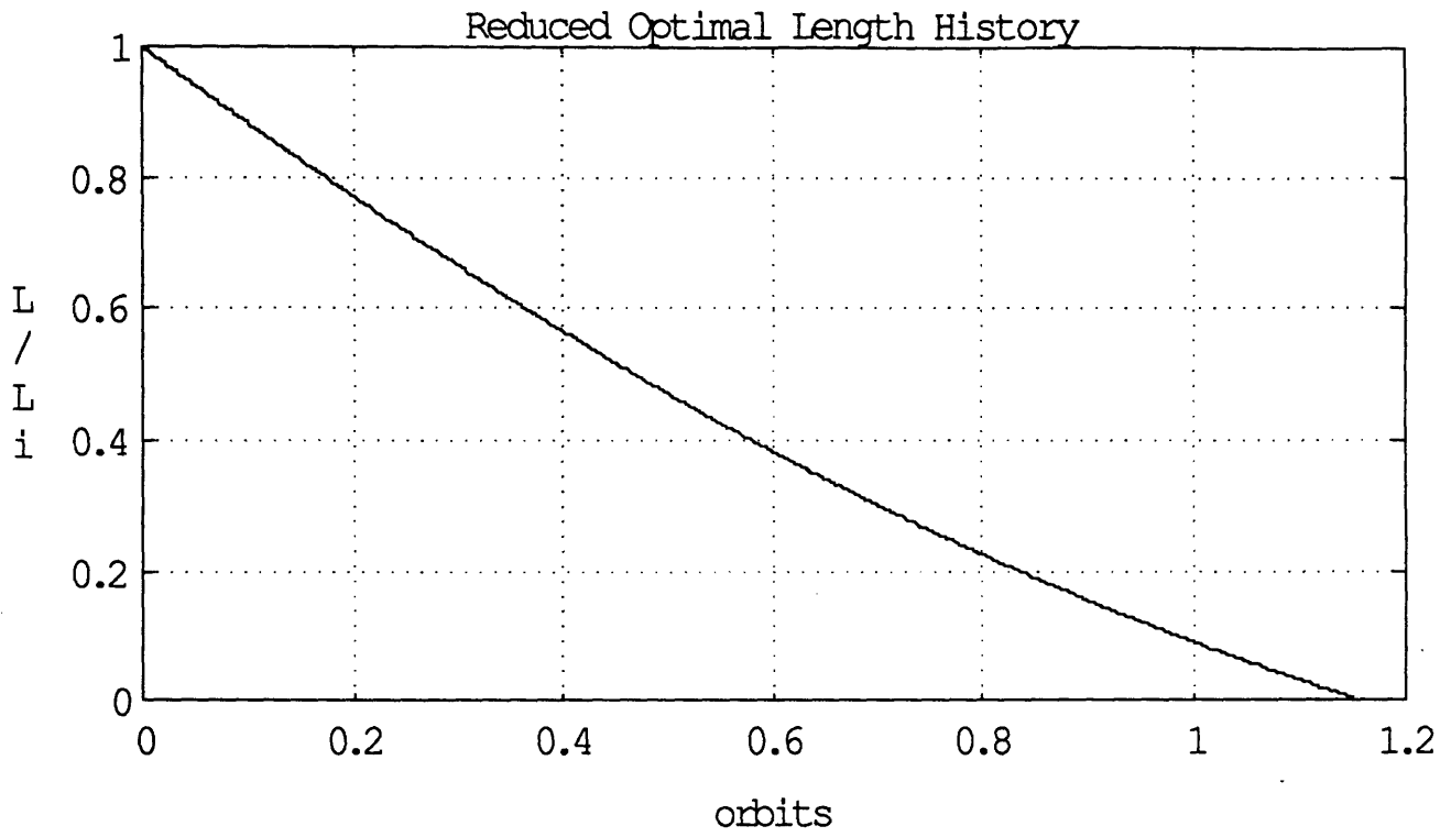
fig 2.11.3: Length history along the reduced optimal trajectory.
