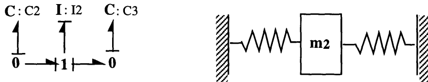
Figure 5.16: Case 2: high frequency oscillation modes.
