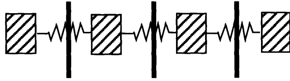
Figure 5.4: The highest frequency oscillation mode of a mass-spring system.
