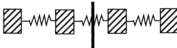
Figure 5.3: The first oscillation mode of a mass-spring system.
