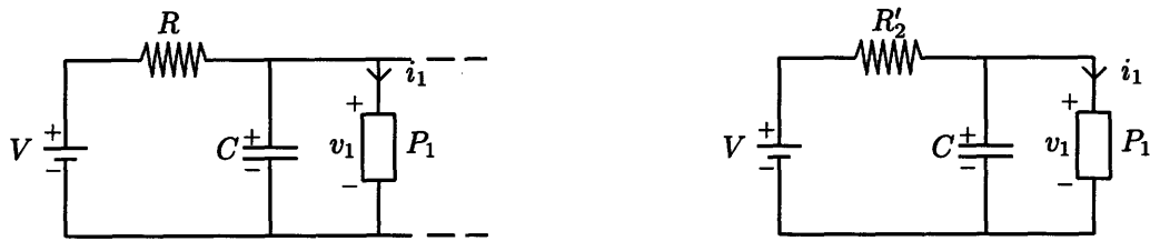
Figure D-4: Example loop with equivalent circuit.
