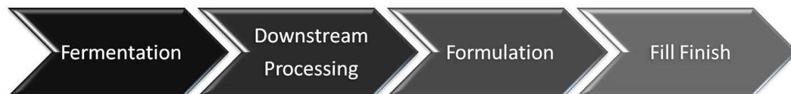
Figure 11-2: Schematic of Biologics Manufacturing
