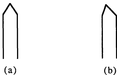
Figure 12. End-on view of scalpel blade: (a) centered cutting edge, (b) off- center cutting edge. [As seen with SEM.]
