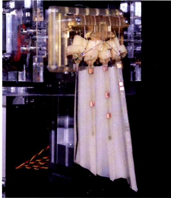
Figure 8. 4-ray biorobotic fin prototype. Tendons at the top actuate the fin rays, which are co-molded and clamped into the urethane fin surface (Photo by James Tangorra).
