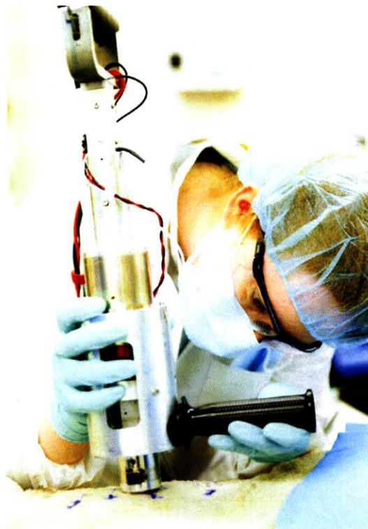
Figure 29. The Bioinstrumentation Lab LLA powered NFI prototype in use on a sedated sheep (Reproduced from Brian Hemond SM2005).
