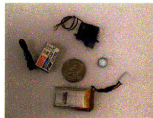
Figure 4-3: Electronics and components: (clockwise from top) hobby servo, motion capture marker, battery, micro receiver.
