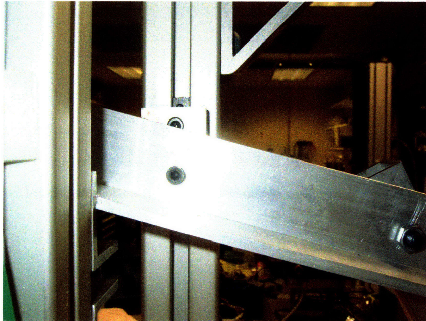
Figure 5-9: "Inside" view of linkage; mating bracket pivot
