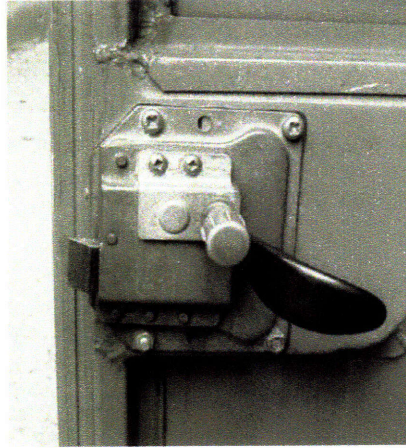
Figure 2-4: Example of simple slam latch on 1970 Land Rover 4
