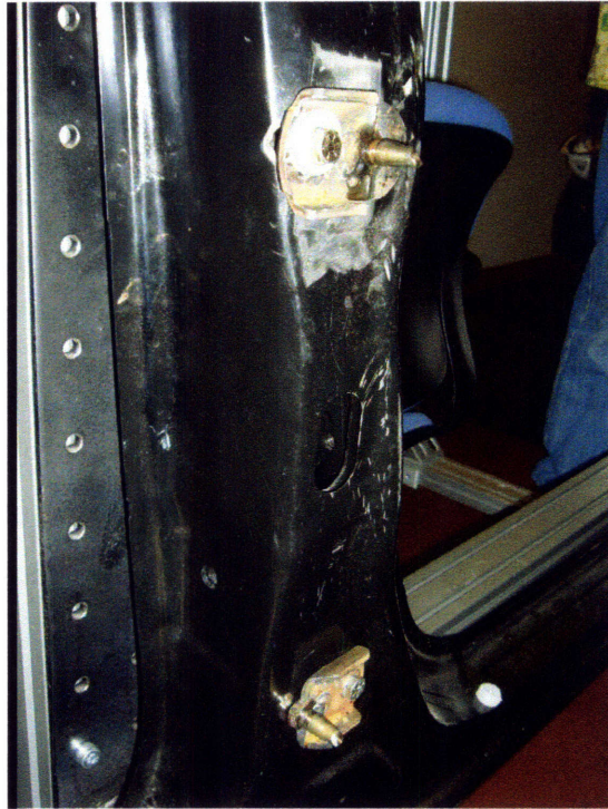
Figure 3-9: Two sets of hinges and plugs bolted to car frame
