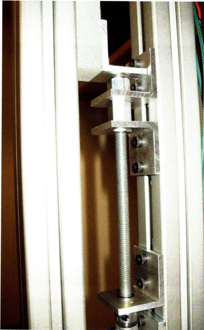
Figure 4-20: Close-up of top hexagonal nut engaged with mating bracket
