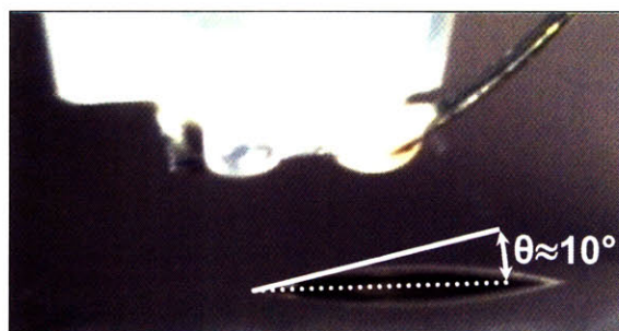
Figure 13. Advancing contact angle measurements of 2-methoxyethanol on platinum.
