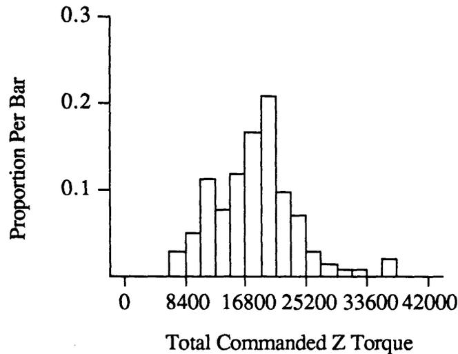
Figure A.15 - Distribution of Integrated Z-Commands (in 20\*N·m·s)
