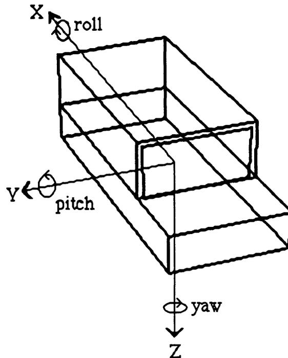
**Figure 2.5 - Simulated-Vehicle Axis Definitions**
