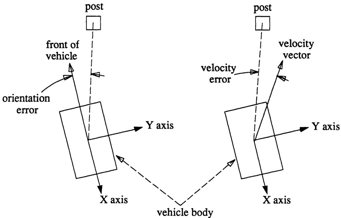
**Figure 3.12 - Orientation Error and Velocity Error Definitions**
