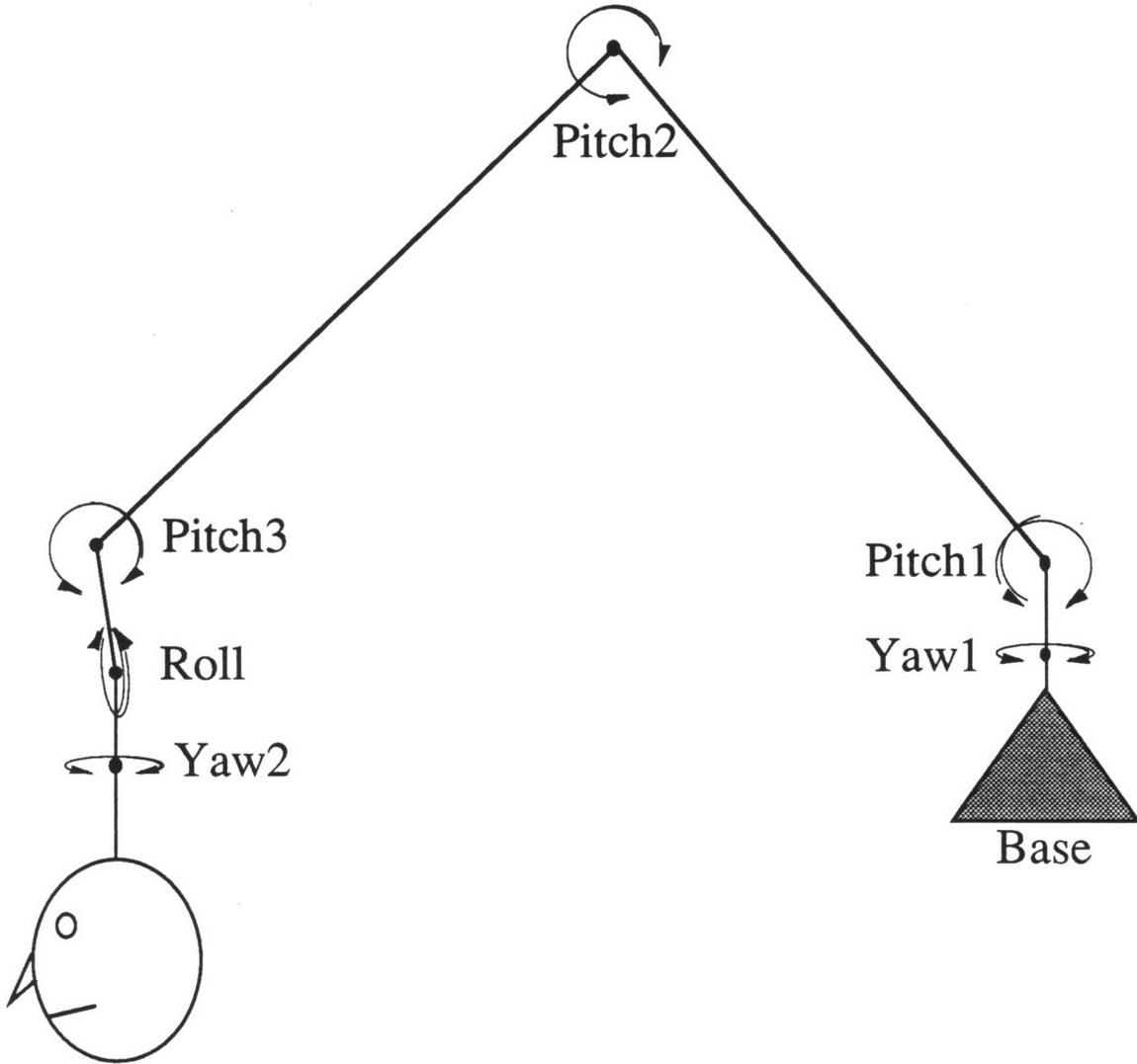
**Figure 2.2 - Head-Tracker Joint Arrangement**
