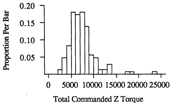
**Figure A.28 - Distribution of Integrated Z-Commands (in 20\*N·m·s)**
