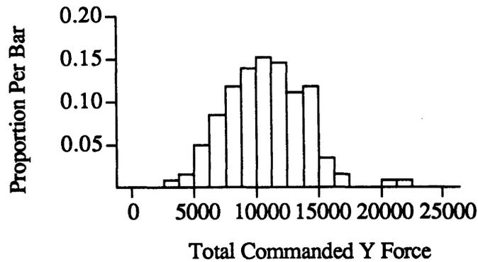
**Figure A.26 - Distribution of Integrated Y-Commands (in 20\*N·s)**
