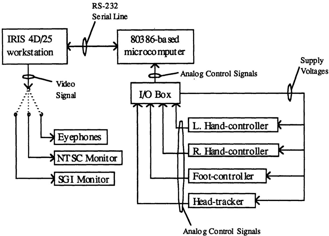
**Figure 2.1 - Block Diagram of Teleoperator Simulation System**
